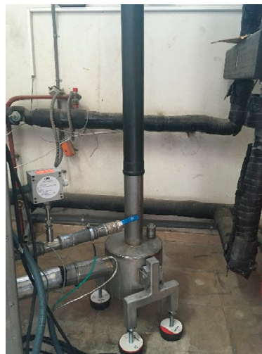
Figure 7. Gas treatment section.
