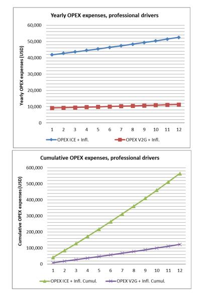
Figure 3. Yearly and cumulative OPEX expenses between an ICE vehicle and a V2G, professional drivers.
