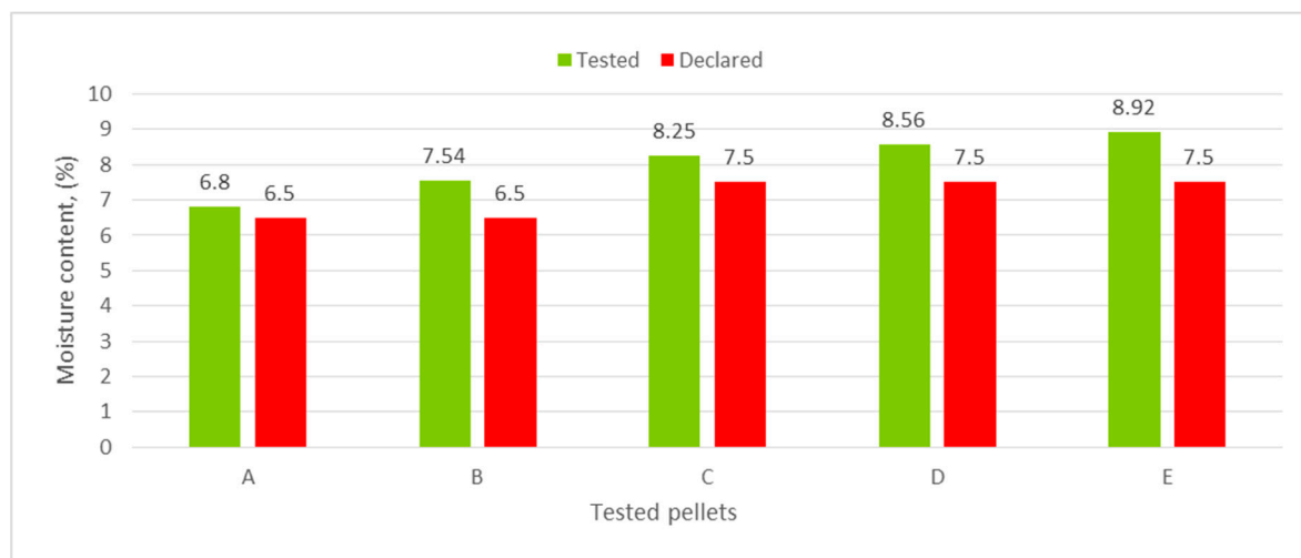
Figure 3. Comparison of the average moisture content in the samples and values declared by the producers printed on the packaging.
