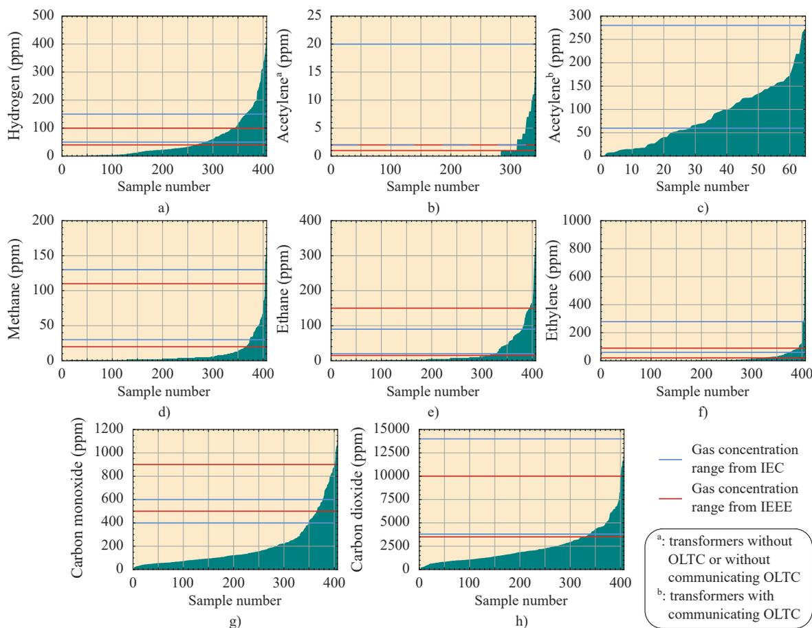
**Figure 3.** Gas concentration data: (a) hydrogen; (b) acetylene (transformers without OLTC or without communicating OLTC); (c) acetylene (transformers with communicating OLTC); (d) methane; (e) ethane; (f) ethylene; (g) carbon monoxide; and (h) carbon dioxide.
