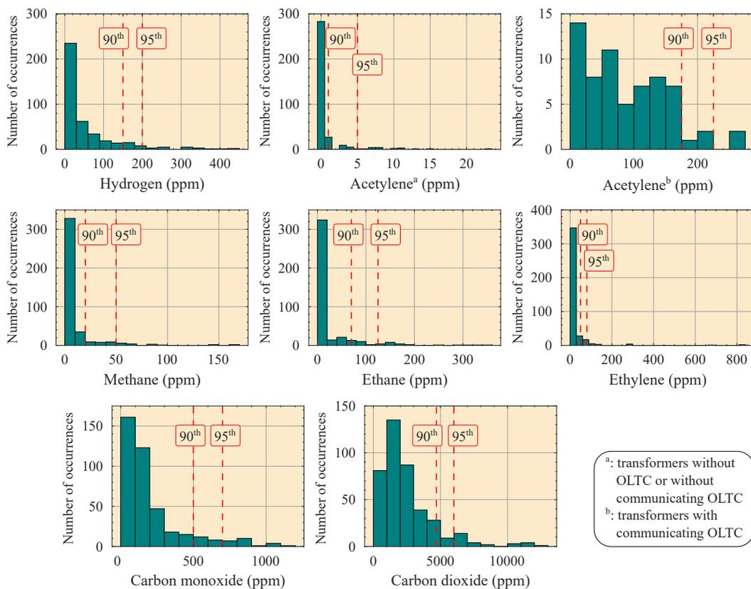
**Figure 4.** Distribution of gas concentrations and calculated 90th and 95th percentiles: (a) hydrogen; (b) acetylene (transformers without OLTC or without communicating OLTC), (c) acetylene (transformers with communicating OLTC); (d) methane; (e) ethane; (f) ethylene; (g) carbon monoxide; and (h) carbon dioxide.
