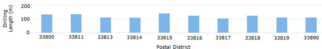
Figure 9. 100 m 2 building in Cangas del Narcea. Drilling length required for each postal district.
