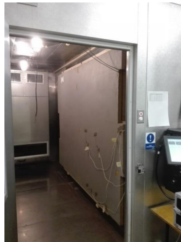
Figure 5. Measured variant B sample on the exterior side of the structure.
