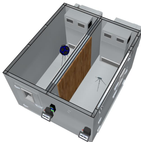
Figure 6. Location of measuring instruments for examining acoustic parameters in the climate chamber.
