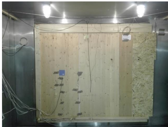
Figure 3. Locations of sensors on the interior side of the structure.
