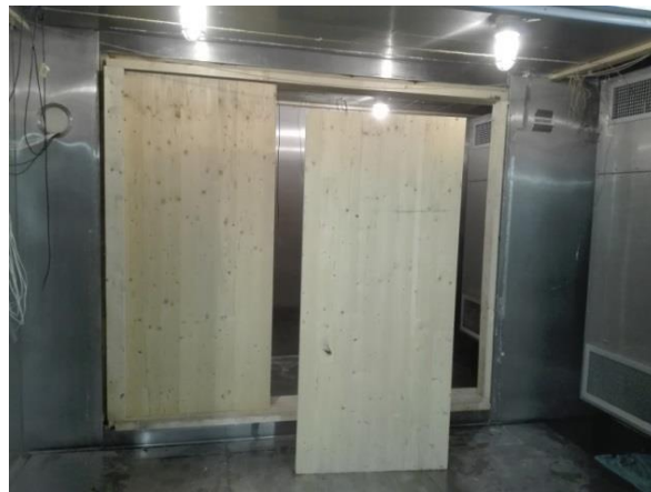
Figure 2. Prefab cross laminated timber structure.
