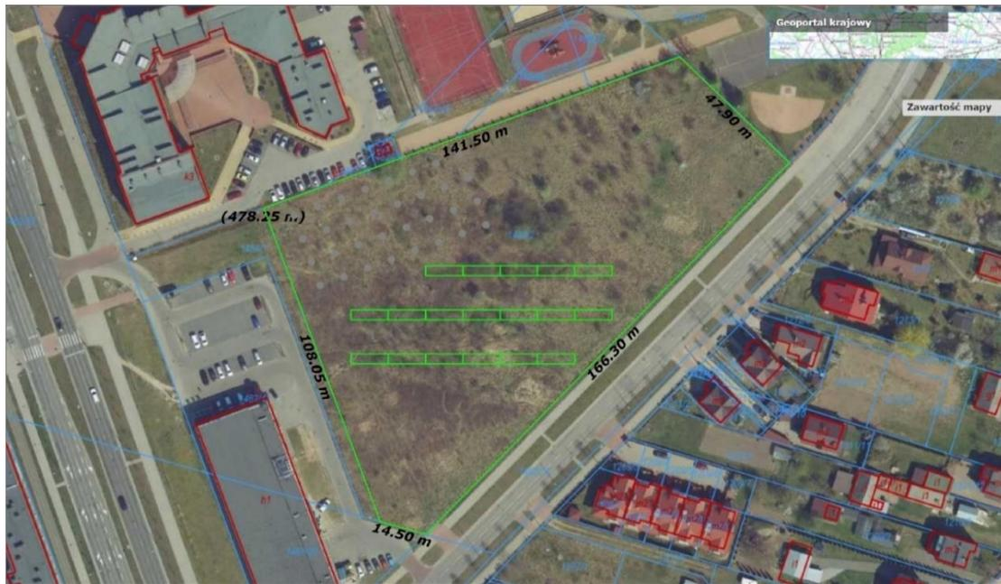
**Figure 7.** Placement of  $4 \times 7$  photovoltaic panels on a neighbouring plot.
