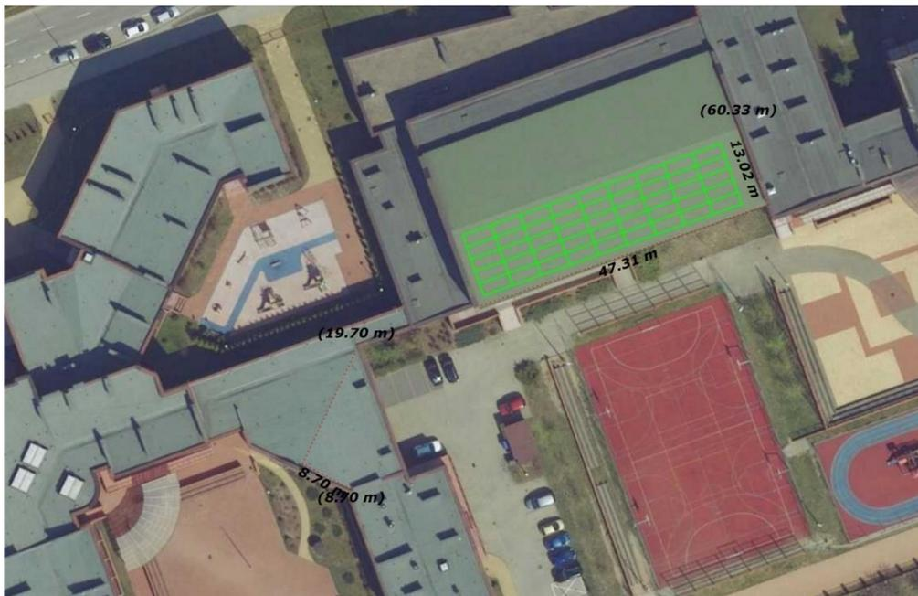
Figure 9. Arrangement of solar collectors on the roof (45 pcs).
