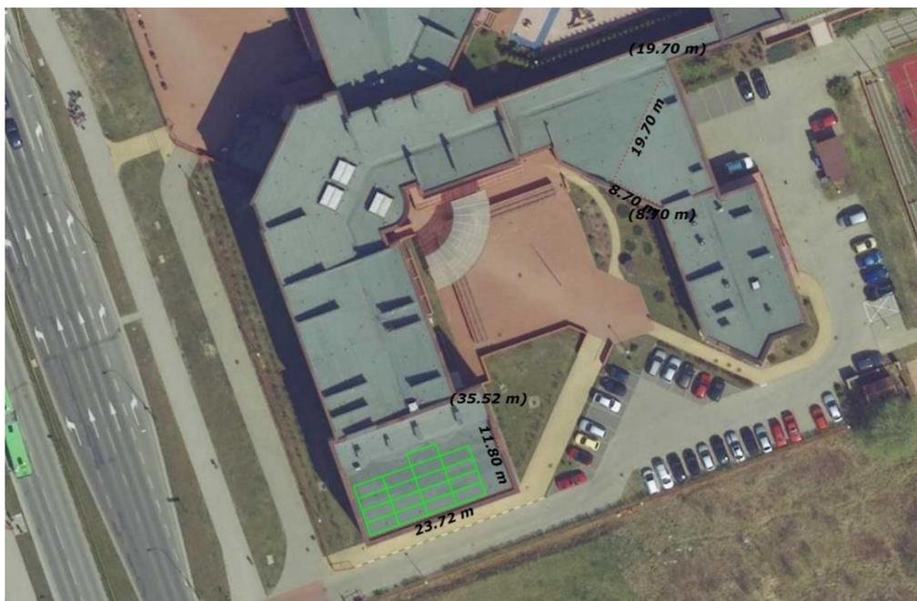
Figure 10. Arrangement of solar collectors on the roof (17 pcs).
