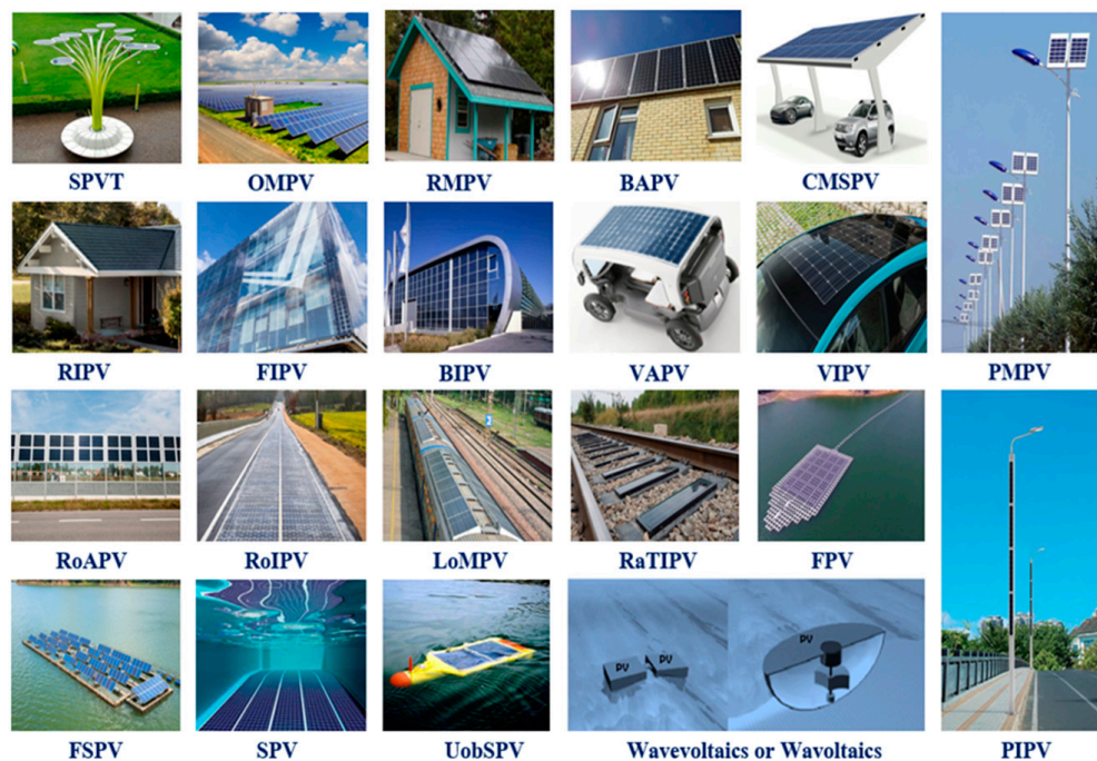
Figure 1. Visual representation of different types of solar photovoltaic plants based on the installation and mounting area. SPVT = solar photovoltaic tree; OMPV = open-mount photovoltaics; RMPV = roof-mount photovoltaics; BAPV = building attached photovoltaics; CMSPV = canopy-mounted solar photovoltaics; RIPV = roof-integrated photovoltaics; FIPV = façade-integrated photovoltaics; BIPV = building-integrated photovoltaics; VAPV = vehicle attached photovoltaics; VIPV = vehicle-integrated photovoltaics; RoAPV = road-attached photovoltaics; RoIPV = road-integrated photovoltaics; LoMPV = locomotive-mount photovoltaics; RaTIPV = rail track integrated photovoltaics; FPV = floating photovoltaics or floatovoltaics; FSPV = floating solar photovoltaics; SPV = submerged photovoltaics; UobSPV = underwater on-board solar photovoltaics; PMPV = pole mounted-photovoltaics; PIPV = pole-integrated photovoltaics.
