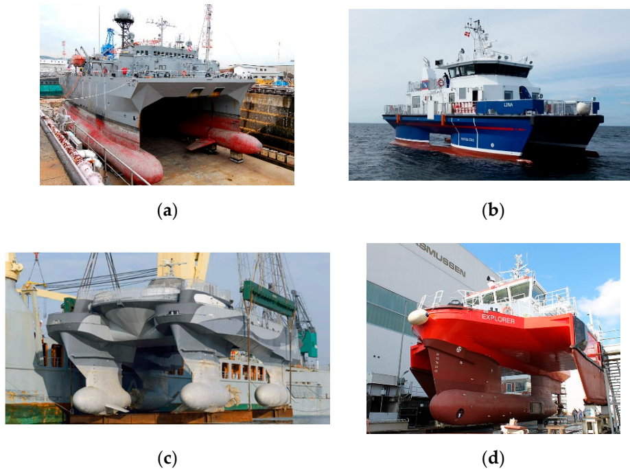
Figure 2. Sample photos of SWATH ships: (a) SWATH GEN. I [46], (b) SWATH GEN. II [47], (c) SWATH GEN. III [48], (d) SWATH GEN. IV-SWASH [49].
