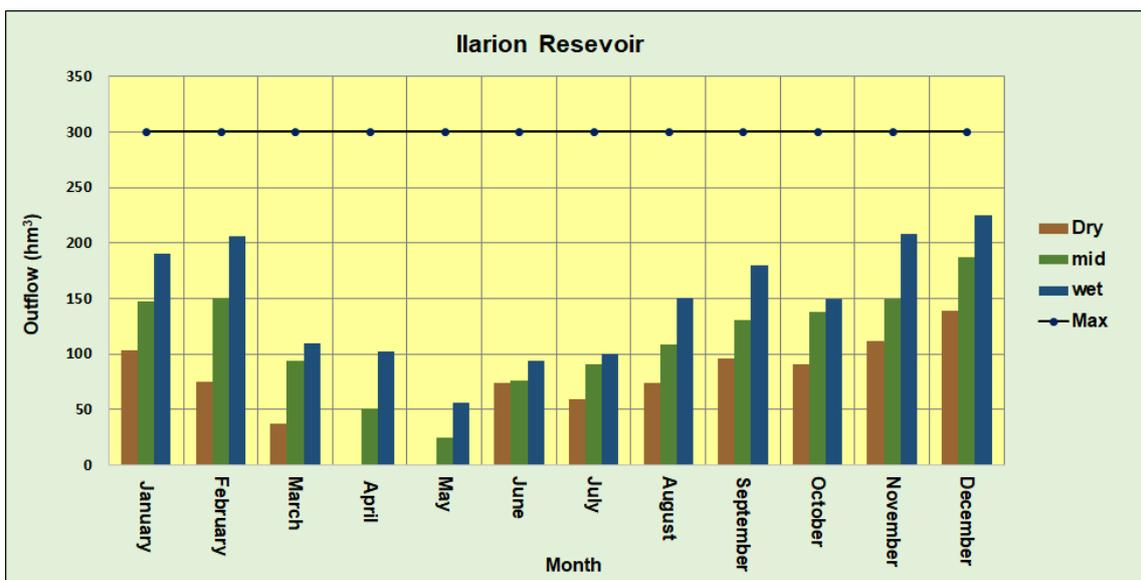
Figure 12. The optimal outflows for the current state of water resources demand, applying the institutional operating rule curves for the Ilarion reservoir.
