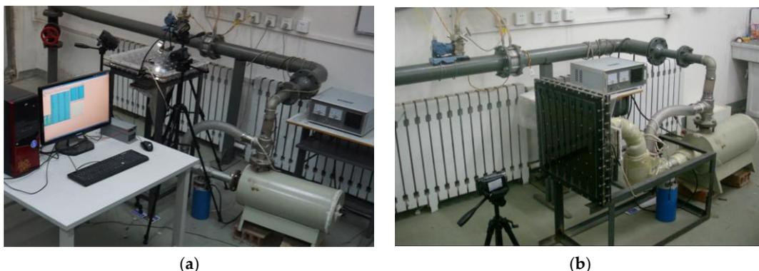
**Figure 2.** Images of test rigs. (a) Test rig of the pin fins. (b) Test rig of the target surface.
