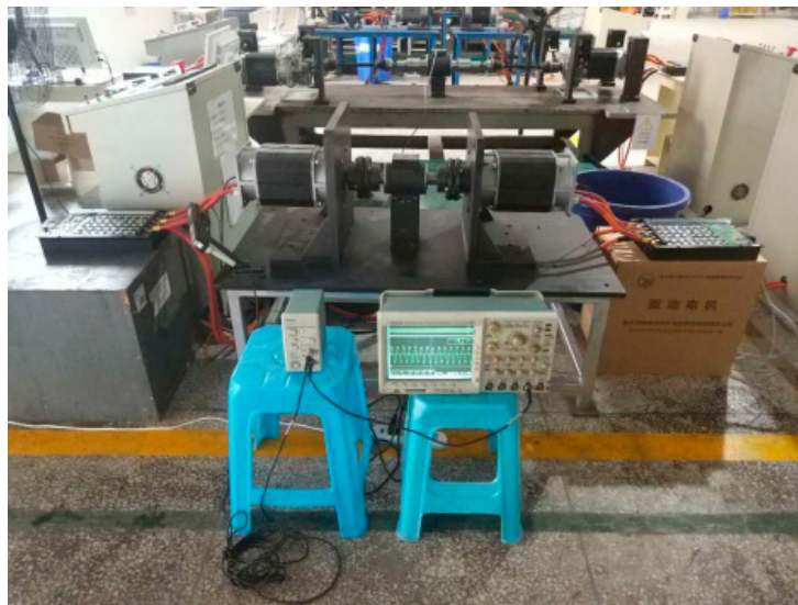
Figure 7. Experiment platform of the 48 V IM drive system.
