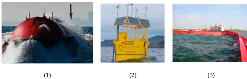
Figure 5. Types of devices studied: Pelamis (1) [62], AquaBuoy (2) [63] and Wave Dragon (3) [64].
