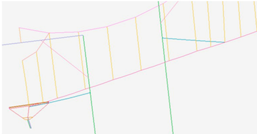
Figure 9. The finite element model of the pantograph catenary system for the trolley wire overhead electrically actuated LHD.
