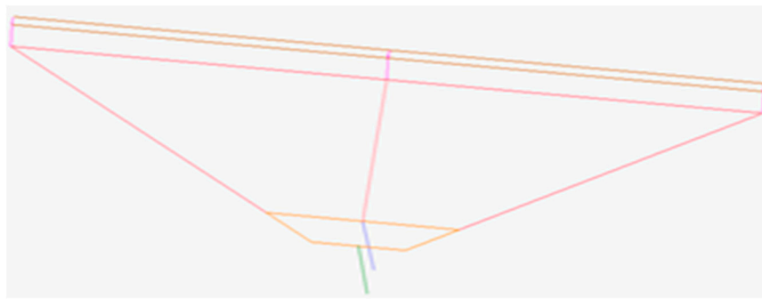
Figure 6. The finite element model of the pantograph system in the pantograph catenary system for trolley wire overhead electrically actuated LHD.
