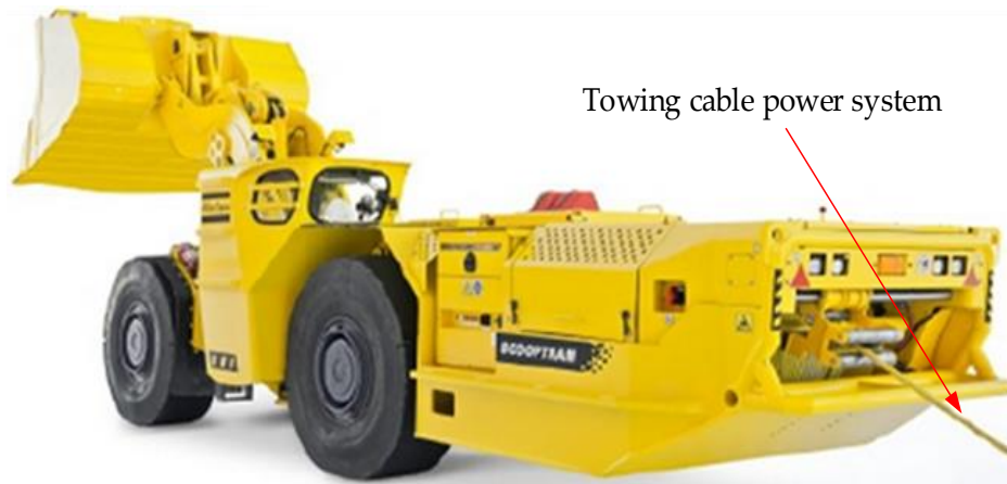
Figure 1. Towed cable electrically actuated load, haul, dump machine (LHD).
