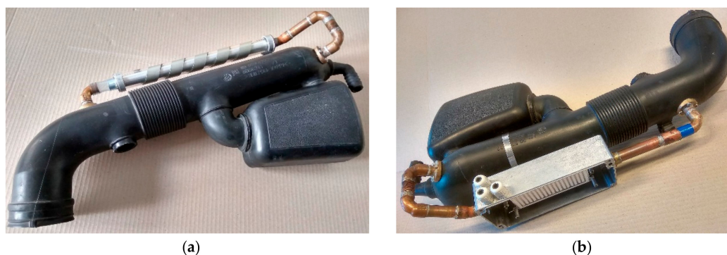
Figure 3. Hardware approach to process automotive engine intake air using manifold by-pass and non-thermal plasma/ozone generated in: (a) volume DBD, (b) SDBD.
