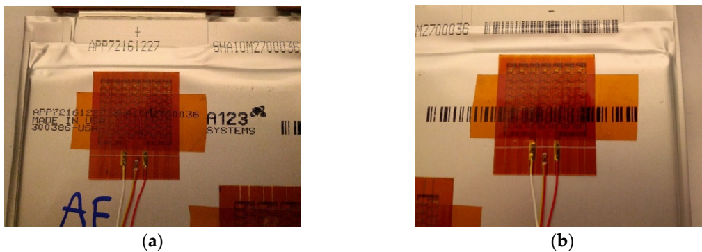
Figure 3. Heat flux sensors locations near (a) cathode and (b) anode.
