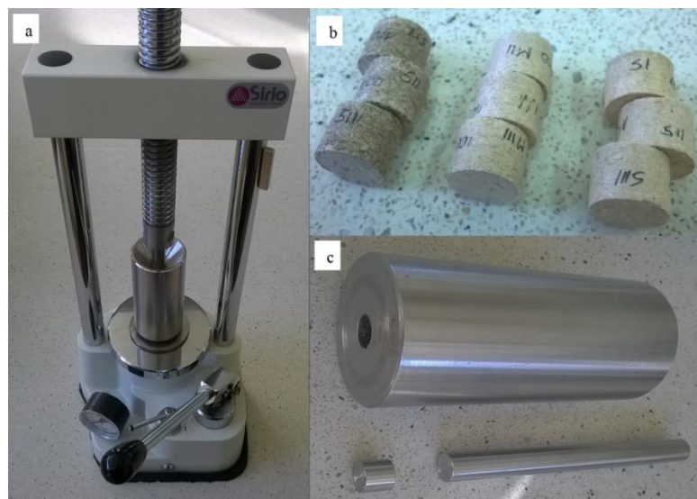
Figure 4. Lab-scale compaction stand for test pellets production: (a) hydraulic press, (b) samples of compacts, and (c) die, piston and bottom.
