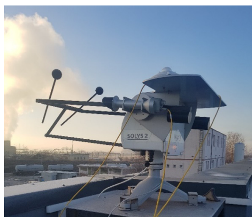
Figure 20. Solys2 solar detection station.
