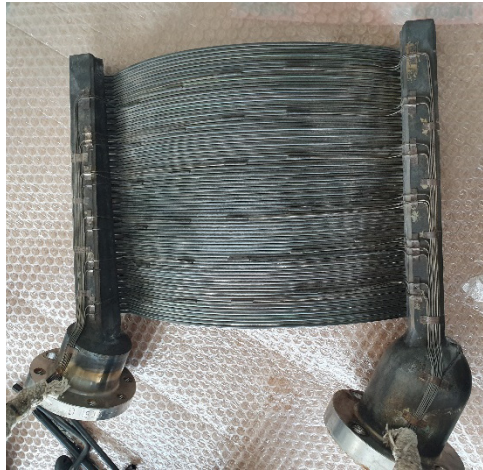
Figure 14. Positioning of temperature sensors on the primary exchanger.
