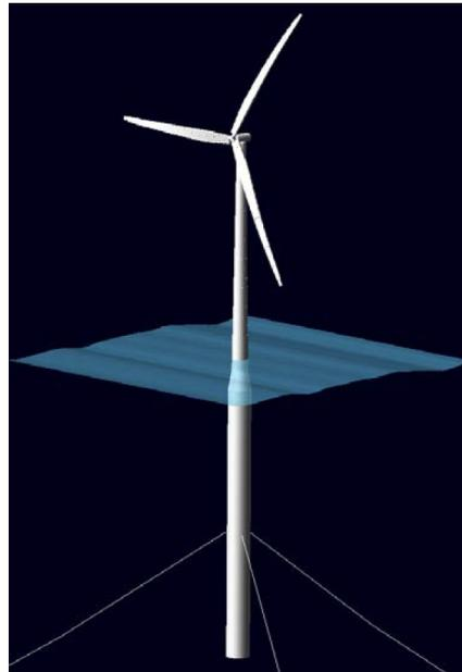
**Figure 2.** Model of the OC3 spar-buoy floating offshore wind turbine (FOWT) system; Reprint with permission [8]; 2010, NREL.
