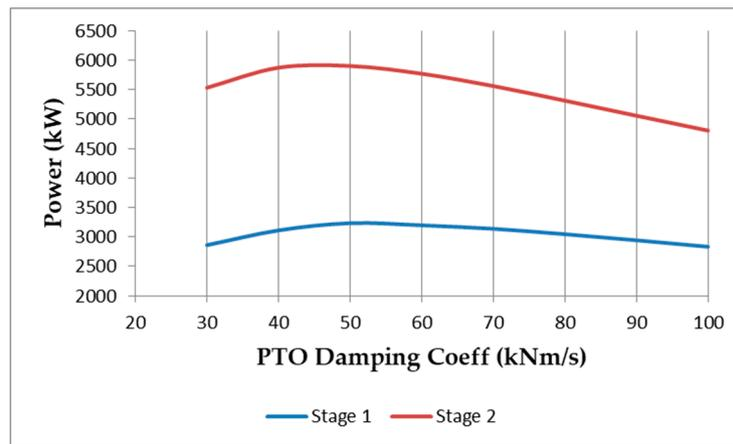
Figure 6. PTO damping vs. power capture.
