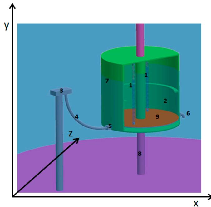
**Figure 1.** The conceptual design of the self-adjusted WEC with main components: 1. Cable/spring; 2. WEC chamber; 3. wave period measuring device and inlet valve to allow seawater flow into the flexible pipe through gravity; 4. flexible pipe; 5. WEC chamber inlet; 6. WEC chamber outlet; 7. WEC buoy; 8. frame; and 9. plate/diaphragm.
