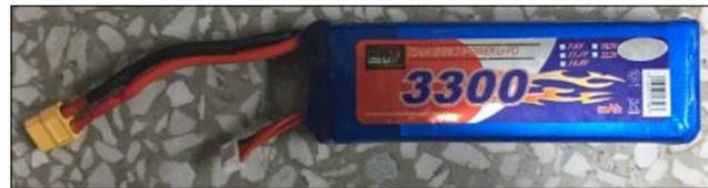
**Figure 6.** Overview of the LiPo battery pack.
