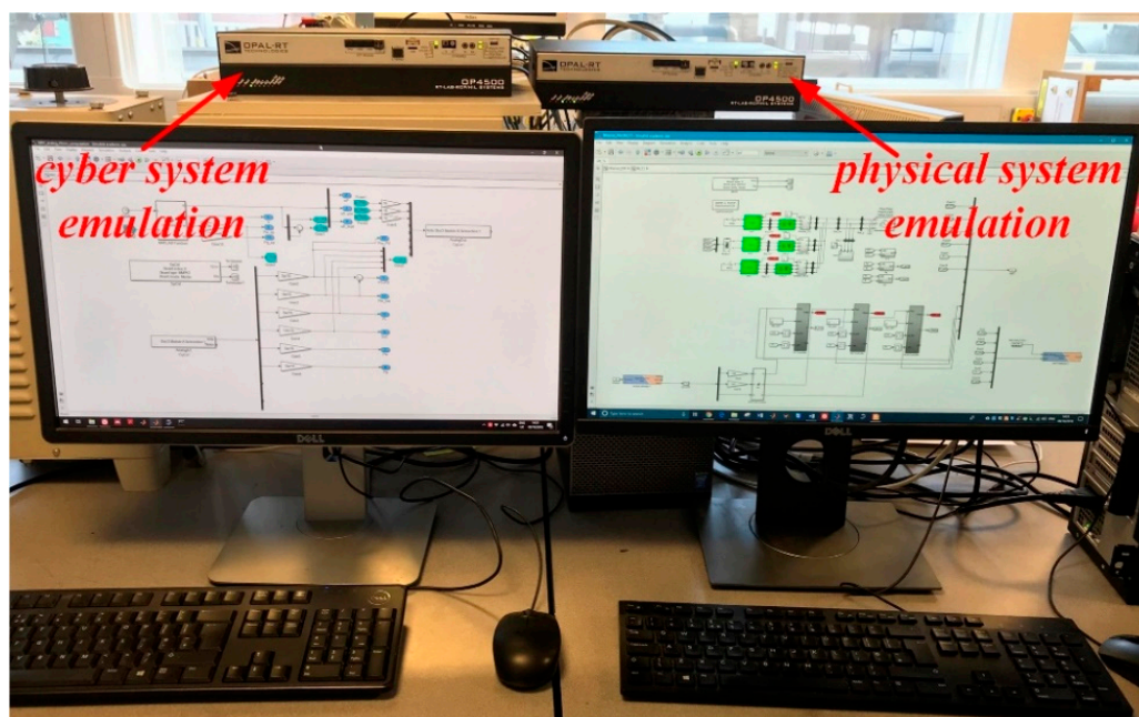
Figure 10. Cyber-physical testbed (co-simulation framework).
