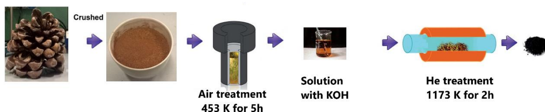
Figure 1. Schematic procedure for the preparation of the activated porous carbons from pinecones.
