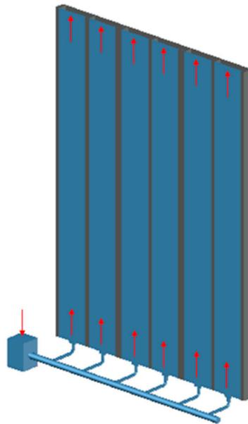
**Figure 2.** Functional scheme of the opaque ventilated façade.
