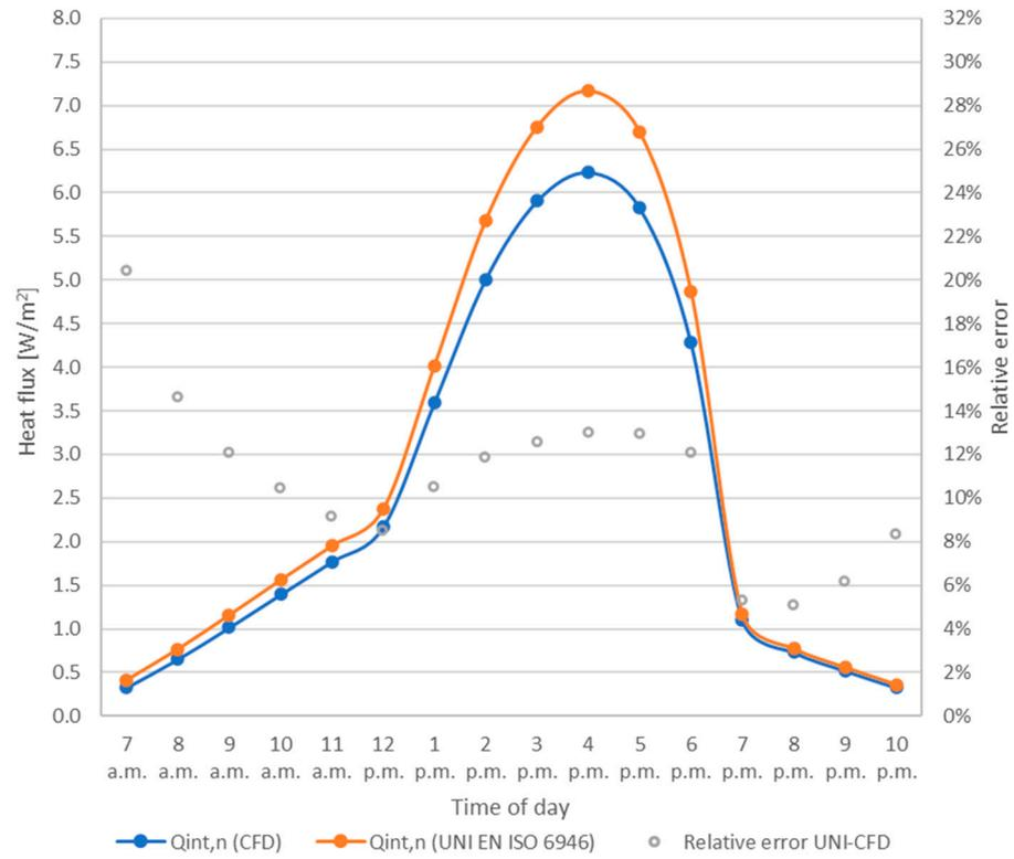
**Figure 10.** Comparison between the heat flux  $Q_{int,n}$  obtained from the CFD analysis and the one calculated following the UNI EN ISO 6946 procedure referred to a well-ventilated air layer. The figure shows also the RE of the CFD results compared to the mentioned Standard at each hour.
