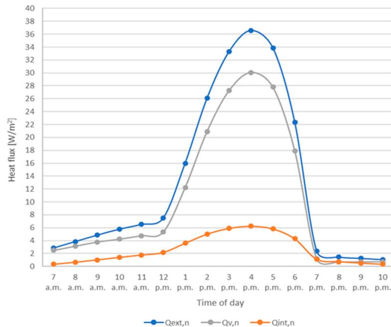
**Figure 8.** Hourly heat flux profiles obtained using the naturally ventilated façade:  $Q_{ext,n}$  is the heat flux coming from the external environment into the cavity,  $Q_{v,n}$  is the one removed by ventilation, and  $Q_{int,n}$  is the heat flux that flows from the cavity to the internal environment.
