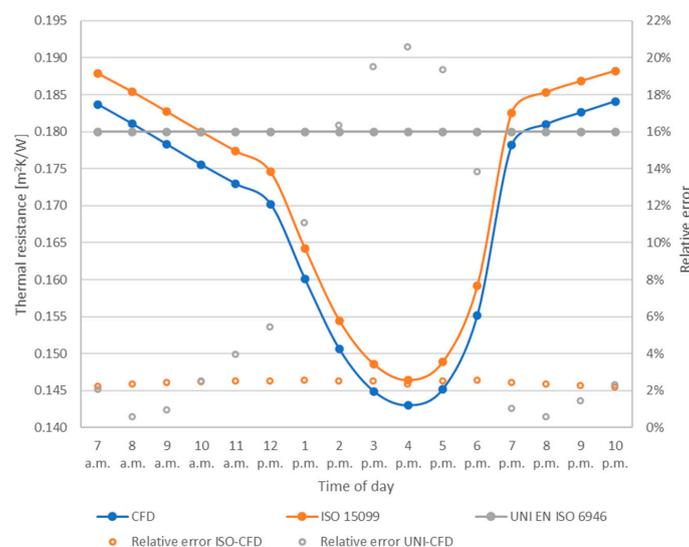
**Figure 5.** Comparison between the hourly thermal resistance values for the closed cavity provided by the CFD simulations and following the ISO 15099 and UNI EN ISO 6946 calculation procedures. The graph shows also the RE of the CFD results compared with the standards at each hour.
