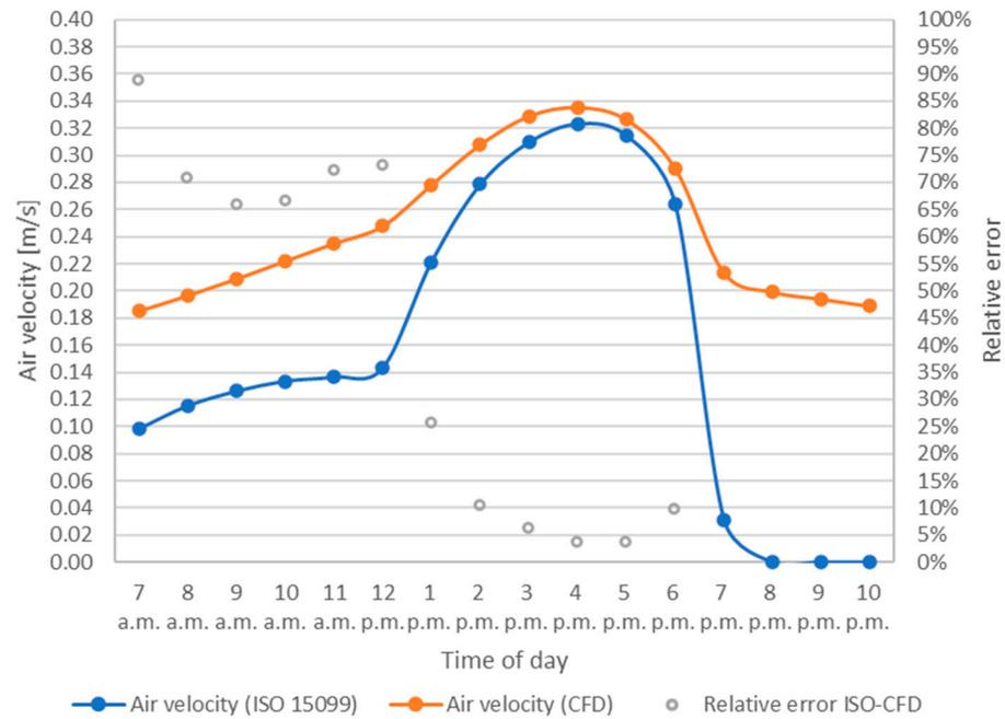
**Figure 12.** Comparison between the average air velocity values inside the naturally ventilated cavity calculated according to ISO 15099 and provided by the CFD simulations. The graph shows also the RE of the CFD compared to the standard, calculated until 6:00 p.m.
