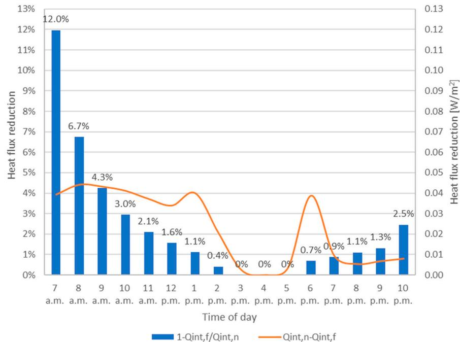
**Figure 9.** Hourly reduction of the heat flux entering the building provided by using forced ventilation ( $Q_{int,f}$ ) instead of natural ventilation ( $Q_{int,n}$ ).
