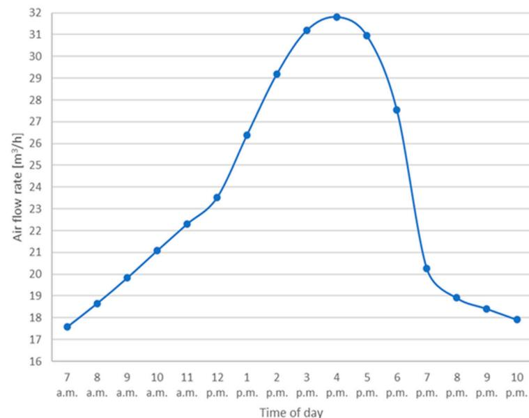
**Figure 7.** Hourly air flow rate through the naturally ventilated cavity.
