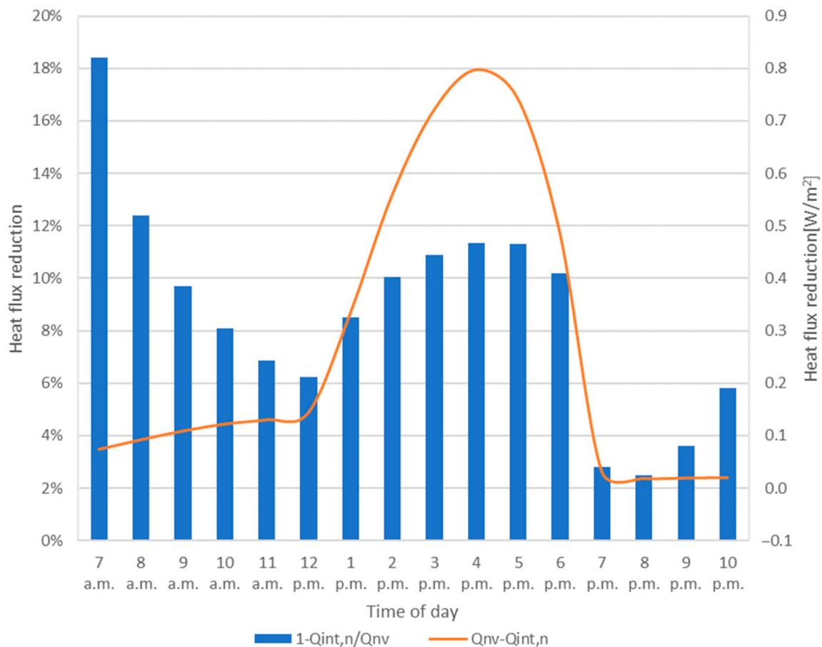
**Figure 18.** Hourly average energy saving ( $S_i$ ) that could be reached using naturally ventilated façade instead of the unventilated one (the chart shows the average  $S_i$  values along the façade height).
