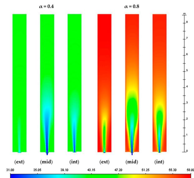
**Figure 16.** Comparison between the temperature profiles (indicated in °C) at 4:00 p.m. on the external (ext) and internal (int) surfaces of the ventilated cavity and on a surface (mid) at half its thickness, considering  $\alpha = 0.4$  and  $\alpha = 0.8$ .
