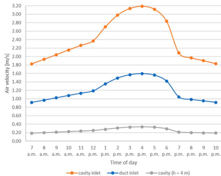
**Figure 6.** Hourly air velocity values referred to: duct inlet section, cavity inlet section (at the bottom of the façade), cross section of the cavity at a height of 4 m.
