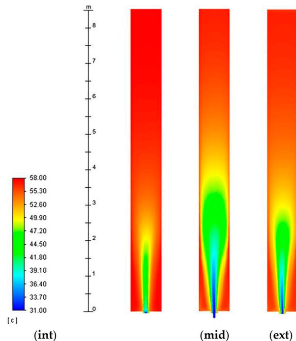
**Figure 15.** Temperature profile inside the naturally ventilated cavity at 4:00 p.m., plotted on the internal (**int**) and external (**ext**) surfaces of the cavity and on another surface (**mid**) at half its thickness.
