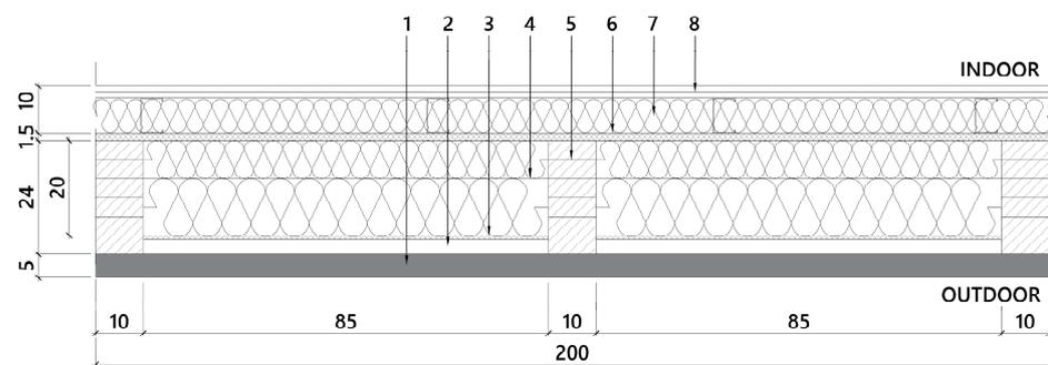
**Figure 1.** Horizontal section of the opaque ventilated façade module analyzed. The layers numbering refers to Table A1.
