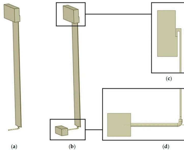
**Figure 3.** Model geometry for forced (a) and natural (b) ventilation. Details (c,d) show respectively the inlet and the outlet domain.
