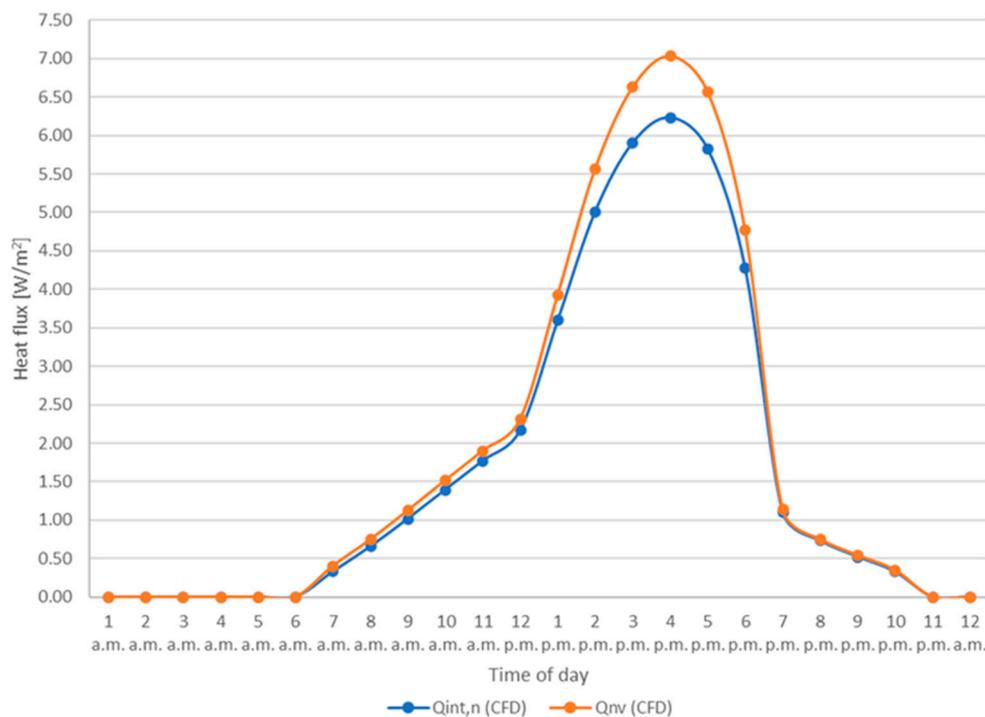
**Figure 17.** Comparison between the heat fluxes entering the building through the naturally ventilated façade ( $Q_{int,n}$ ) and the unventilated façade ( $Q_{nv}$ ).
