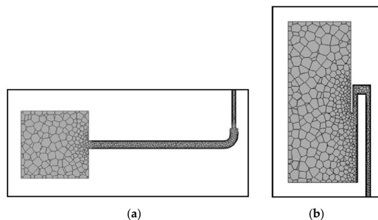
**Figure 4.** Vertical sections of the inlet (a) and outlet (b) volumes mesh.
