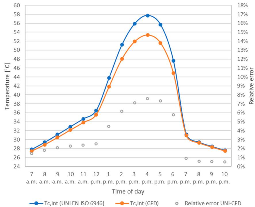
**Figure 11.** Comparison between the temperature values of the internal face of the cavity obtained by UNI EN ISO 6946 and by CFD. The graph shows also the RE of the CFD compared to the standard at each hour.
