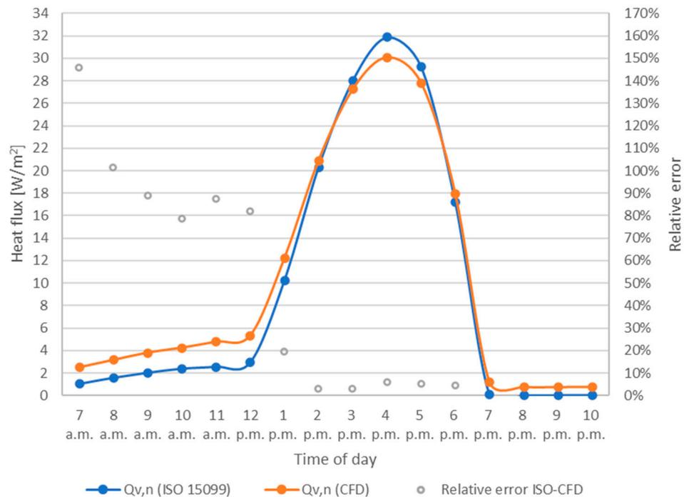
**Figure 13.** Comparison between the heat flux removed from the cavity by natural ventilation ( $Q_{v,n}$ ) calculated according to ISO 15099 and CFD simulations. The graph shows also the RE of the CFD compared to the standard, calculated until 6:00 p.m. local results.
