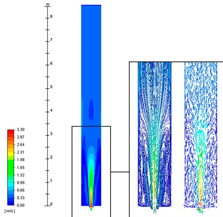
**Figure 14.** Air velocity profile inside the naturally ventilated cavity at 4:00 p.m., plotted on a surface at half the thickness of the cavity.
