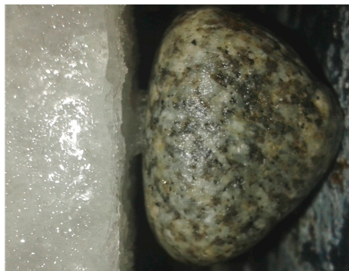
Figure 4. Salt bridge on the contact between salt sample and individual aggregate grain.
