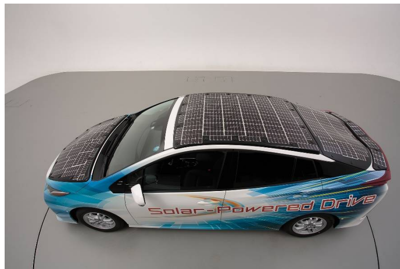
Figure 21. Picture of the Prius Plug-in Hybrid with solar cells [139].
