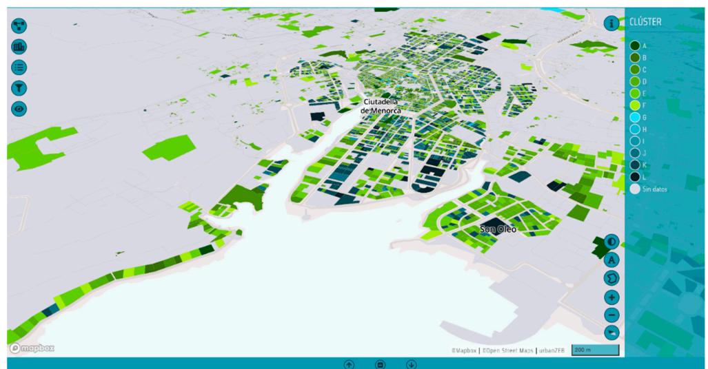
Figure 7. Aerial view showing the filters applied on residential buildings, and presenting the 12 archetypes based on year of construction and typology. Source: urbanZEB web platform.
