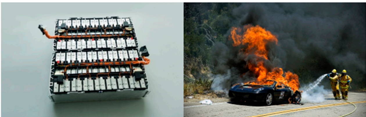
Figure 2. LIB pack applied in an EV (left). LIB in an EV catches fire (right) [8].
