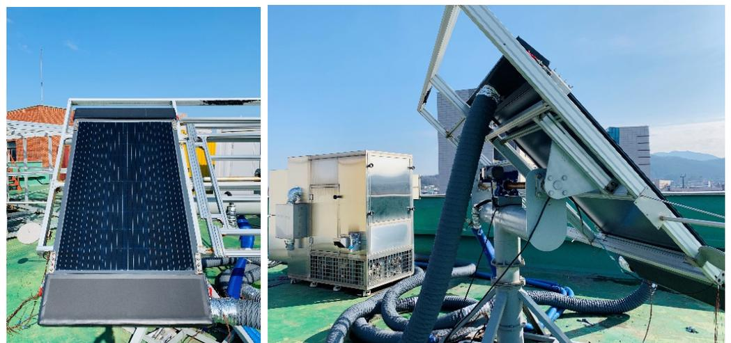
**Figure 3.** Installation for air-type PVT collector Experiment.
