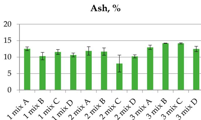
**Figure 4.** The ash content from the combustion of biofuel pellets (proportions of potato and beans: 1:1 (A); 1:2 (B); 1:3 (C); 1:4 (D) by volume).
