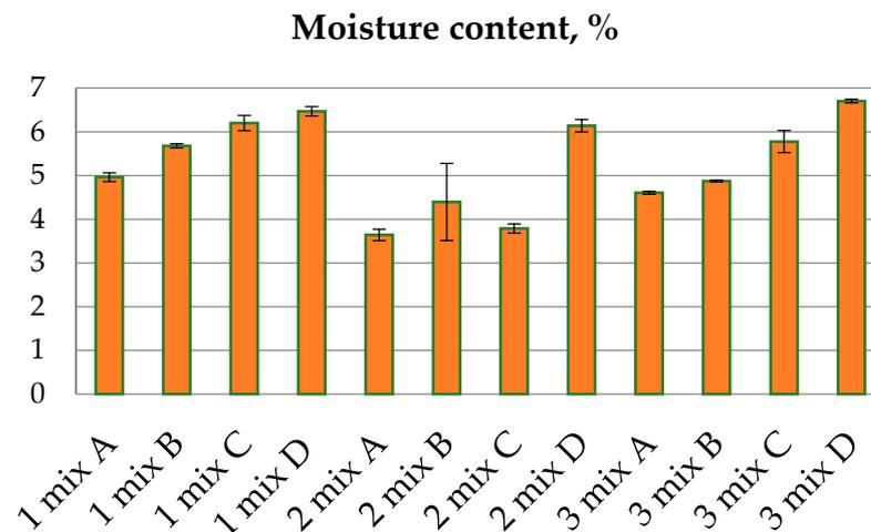
**Figure 2.** Moisture content of pellets, % (proportions of potato and beans: 1:1 (A); 1:2 (B); 1:3 (C); 1:4 (D) by volume).
