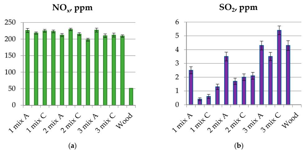
Figure 8. NO<sub>x</sub> (a) and SO<sub>2</sub> (b) emissions from burning of granulated faba bean waste and potato peels.
