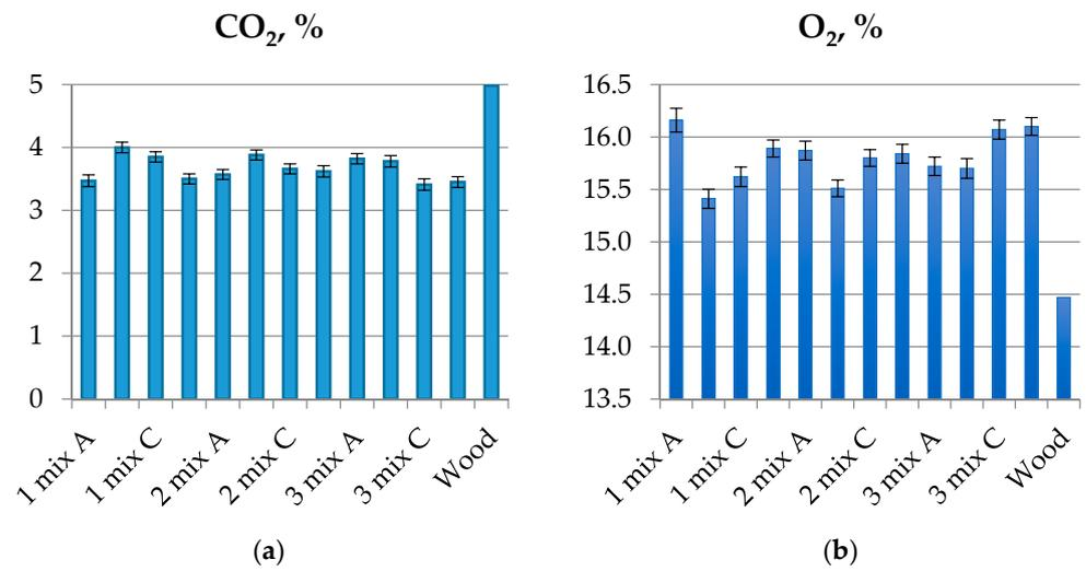
Figure 6. CO<sub>2</sub> (a) and O<sub>2</sub> (b) emissions from burning of granulated faba bean waste and potato peels.
