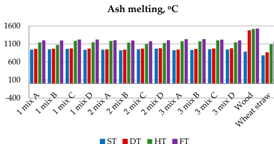
**Figure 5.** Ash melting temperatures of plant waste pellets (proportions of potato and beans: 1:1 (A); 1:2 (B); 1:3 (C); 1:4 (D) by volume).
