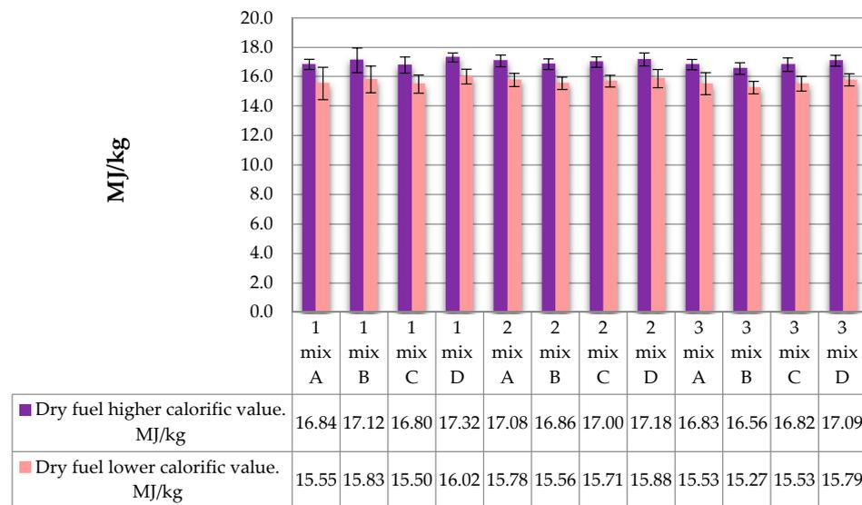
**Figure 3.** Calorific value of faba bean and potato peel pellets (proportions of potato and beans: 1:1 (A); 1:2 (B); 1:3 (C); 1:4 (D) by volume).
