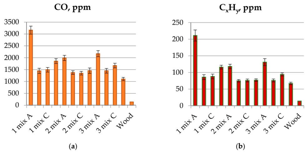
Figure 7. CO (a) and C<sub>x</sub>H<sub>y</sub> (b) emissions from burning of granulated faba bean waste and potato peels.
