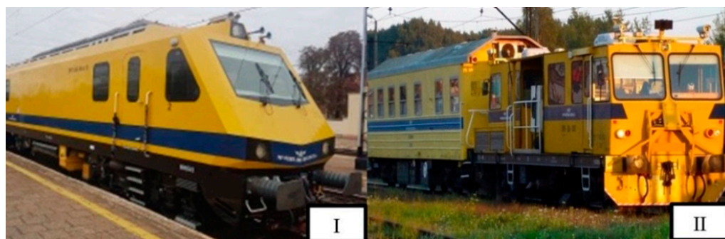
Figure 1. Tested objects: I—track geometry vehicle, II—clearance vehicle.
