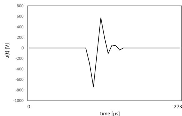
**Figure 6.** Extracted transient using wavelet transform and formula (5).
