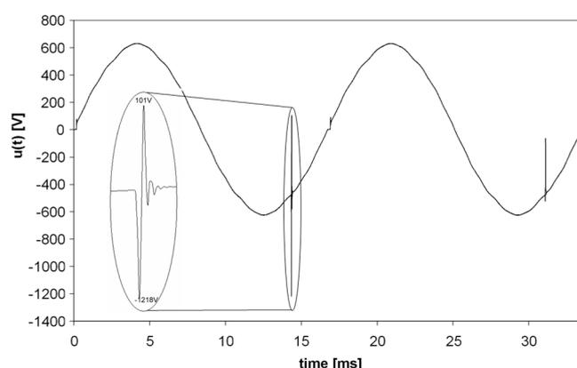
**Figure 5.** Example transient registered in a ship network [55].
