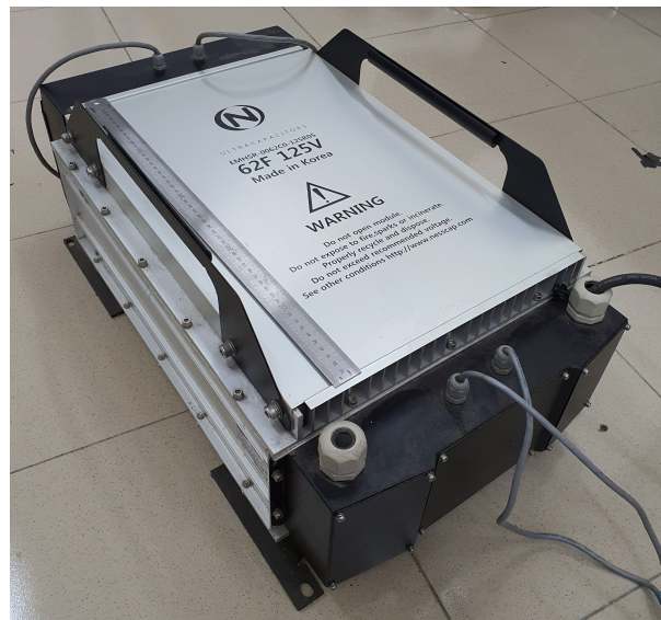
Figure 9. Experimental supercapacitor NESSCAP EMHSR-0062C0-125R0SR2.
