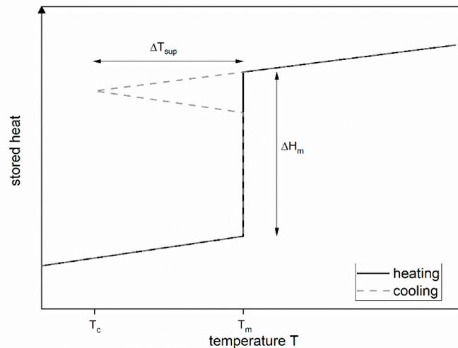
**Figure 1.** Exemplary depiction of the supplied heat above the material temperature with a representation of the melting enthalpy  $\Delta H_m$  and supercooling during the cooling process  $\Delta T_{sup}$ .
