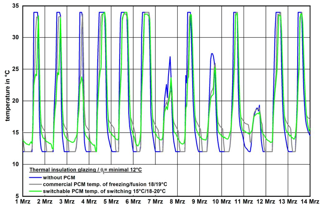
**Figure 8.** Comparison of the time dependence of the indoor air temperatures when using thermal insulation glazing without a PCM (blue), with a commercially available PCM (gray), and with a newly developed, programmable PCM (green), which is activated at an outdoor air temperature of 15 °C.
