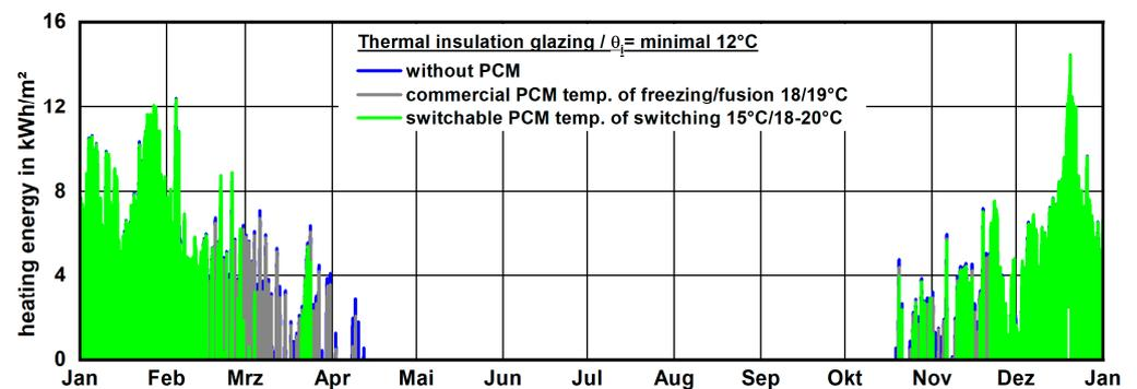
**Figure 9.** Comparison of the required heating energy during a year when using thermal insulation glazing without a PCM (blue), with a commercially available PCM (gray), and with a newly developed, programmable PCM (green).
