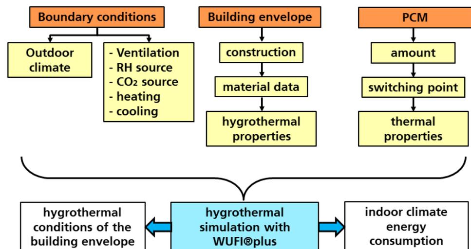
**Figure 5.** Flowchart for carrying out a hygrothermal building simulation using PCMs.
