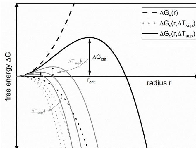
**Figure 2.** Representation of the critical enthalpy difference  $\Delta G_c$  with maximum  $\Delta G_{crit}$  and its dependence on the amount of supercooling  $\Delta T_{sup}$ , as well as on the radius  $r$  of the idealized crystallization nuclei [10].
