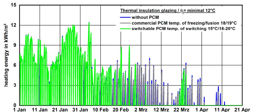
**Figure 10.** Comparison of the required heating energy for the period from 1 January to 21 April when using thermal insulation glazing without a PCM (blue), with a commercially available PCM (gray), and with a newly developed, programmable PCM (green).
