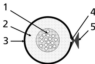
**Figure 3.** Exemplary sketch of the switching mechanism with nucleating agent dispersed in a small portion of the PCM (1), immobilized PCM layer (2), encapsulation layer (3) with a small opening (4), and sealing mechanism (5).
