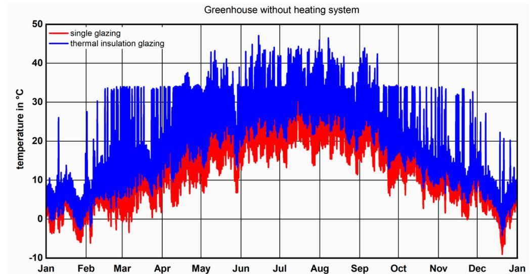
**Figure 7.** Comparison of the time dependence of indoor air temperatures for single (red) and thermal insulation glazing (blue).
