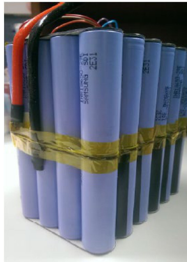
Figure 2. Lithium-ion battery module.
