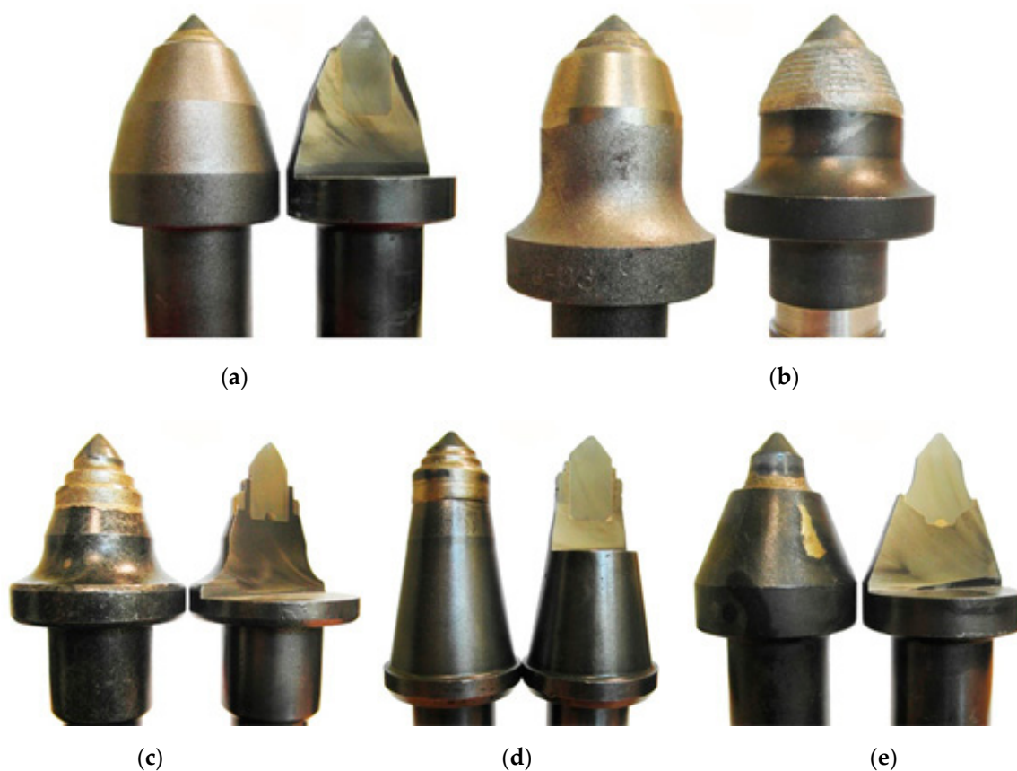
Figure 4. Options of additional protection of conical picks against abrasive wear: (a) standard pick; (b) welded picks; (c) pick with a ring made of WC-Co; (d) pick with two rings made of WC-Co; (e) pick with a lowered body and WC-Co insert in the CAP type [28].
