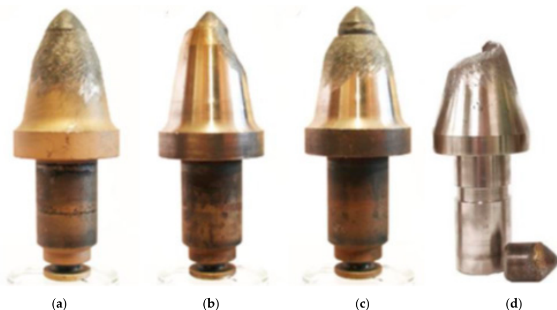
Figure 3. Worn conical picks: (a) properly (symmetrical); (b) improperly (asymmetrical); (c) with the tip exposed; and (d) with the tip falling out [37].
