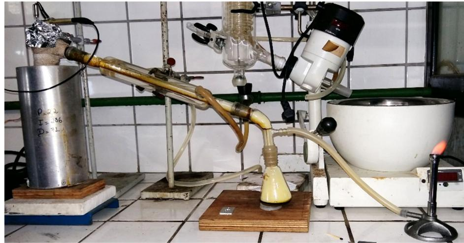
Figure 3. View of the pyrolysis unit in laboratory scale.
