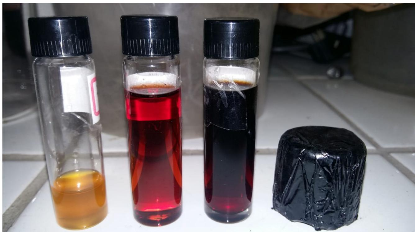
**Figure 9.** Distillation fractions [gasoline (yellow), light kerosene (red), and kerosene (red dark)-like boiling range temperature fossil fuels] and bottoms [Raffinate (black solid)] obtained by fractional distillation of bio-oil produced by pyrolysis of Açai (*Euterpe oleracea*, Mart.) seeds at 450 °C and 1.0 atmosphere, in pilot scale.
