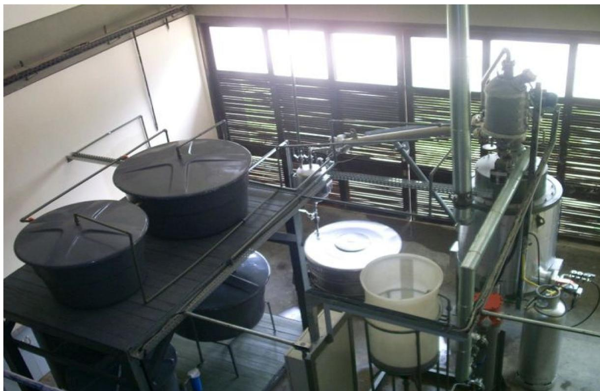
**Figure 5.** View of the pyrolysis unit in pilot scale.
