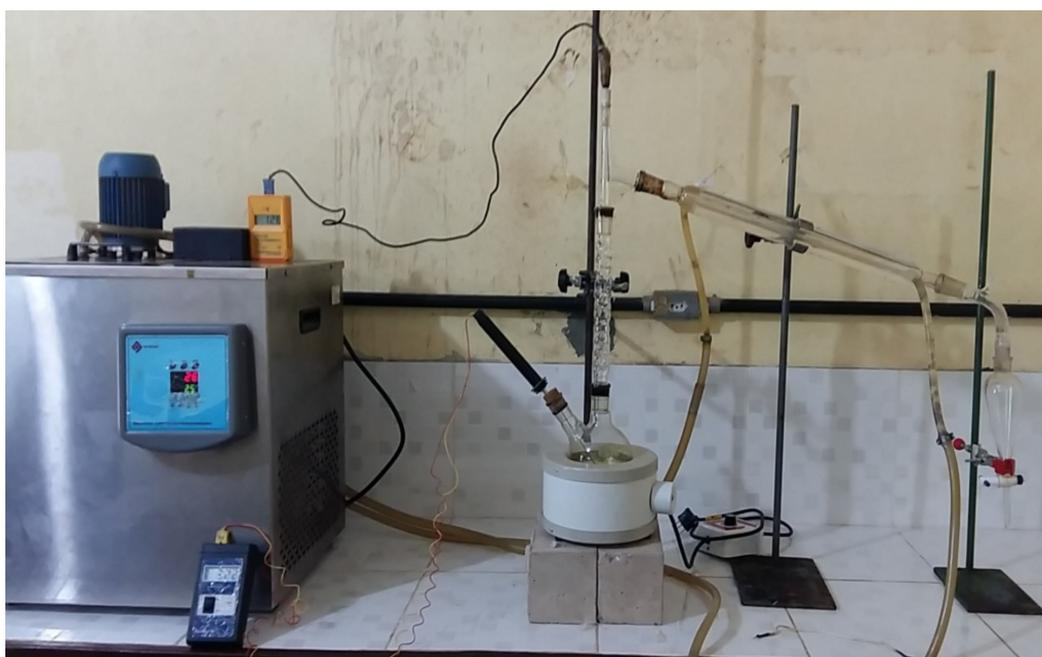
Figure 6. View of distillation column (Vigreux).
