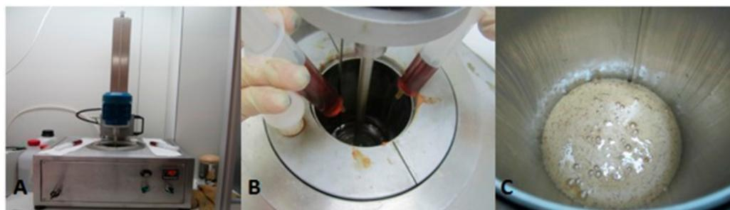
**Figure 2.** Stages of the RPU foam production: (A) synthesis reactor; (B) diisocyanate addition, and (C) foam rising.
