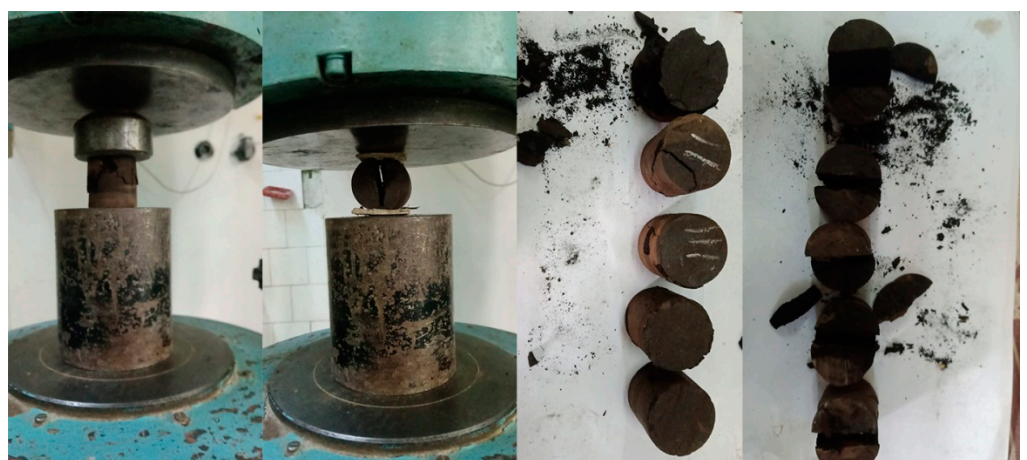
Figure 14. Laboratory testing of lignite samples.
