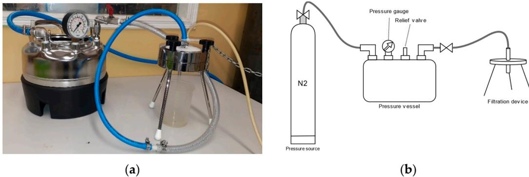
**Figure 1.** Sterlitech pressure filtration vessel: (a) photograph; (b) diagram.
