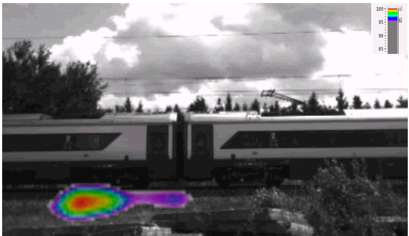
Figure 12. Sound level distribution within a frequency range of 2000–3000 Hz—straight section.
