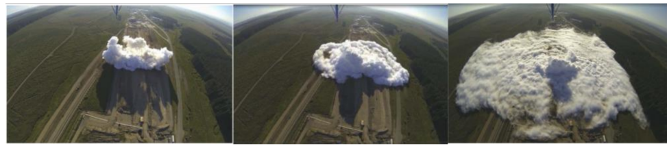
Figure 3. The visible cloud behavior after the rupture; from left to right, at 10, 30 and 120 s from the break (This figures were published from International Journal of Greenhouse Gas Control , Ahmad et al. [40], Copyright Elsevier, 2015).
