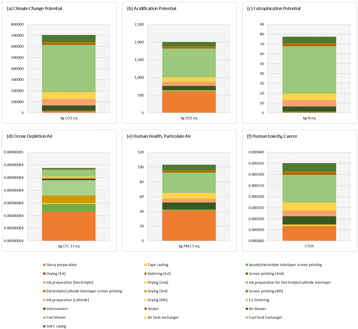
Figure 5. LCA results for six impact categories for the process during the SOFC manufacturing phase.
