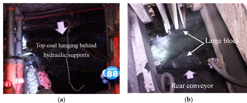
Figure 2. Undesired caving behaviors of top-coal. (a) Delayed caving; (b) formation of the large top-coal block.
