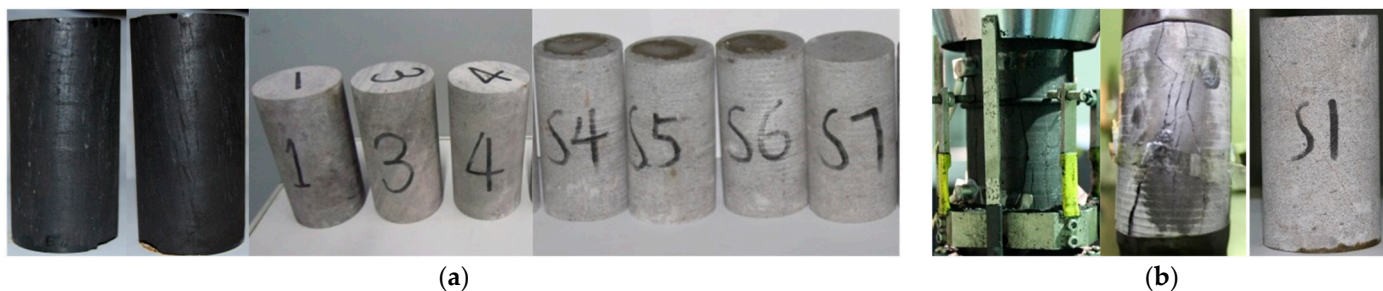
Figure 5. Rock specimens before and after uniaxial compression test. (a) Intact specimens; (b) failure modes.
