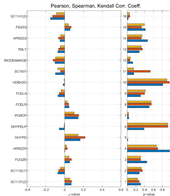
Figure 13. Pearson (yellow), Spearman (red), and Kendall (blue) correlation coefficients for FPT model; H 2 production (final core state) vs. uncertainty parameters. Values for IRODDAMAGE and SC1001 have no meaning.
