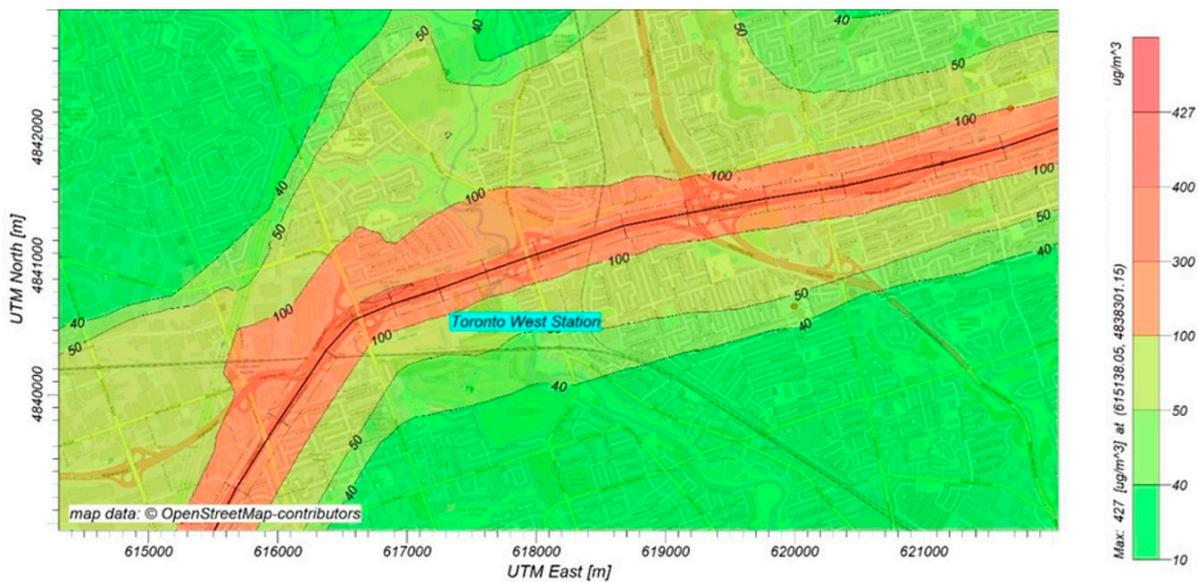
**Figure 11.** Maximum  $\text{NO}_x$  concentration due to traffic in 2017 in vicinity of the West Toronto Air Pollution Monitoring Station ( $\mu\text{g}/\text{m}^3$ ).
