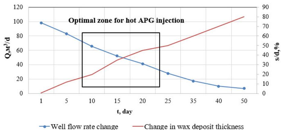
Figure 6. Determination of the optimal hot APG injection period.
