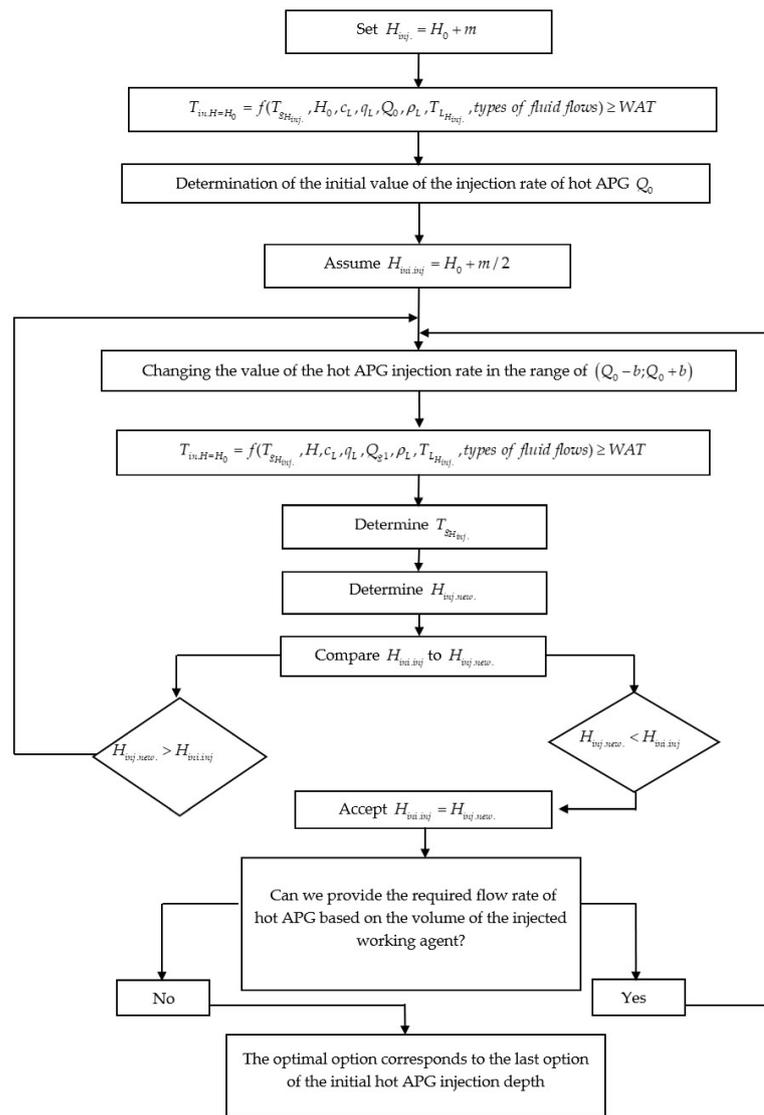
**Figure 5.** Algorithm for determining the optimal injection depth and flow rate of hot associated petroleum gas in a gas-lift well.
