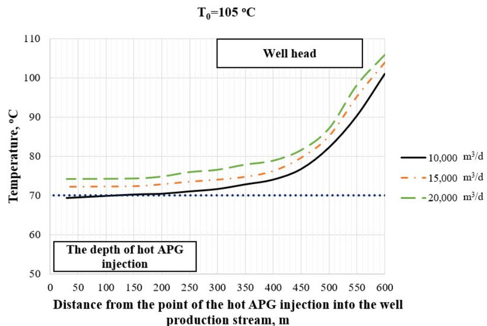
Figure 8. Annulus hot APG temperature profile, inlet  $T_0 = 105 \text{ }^\circ\text{C}$ .
