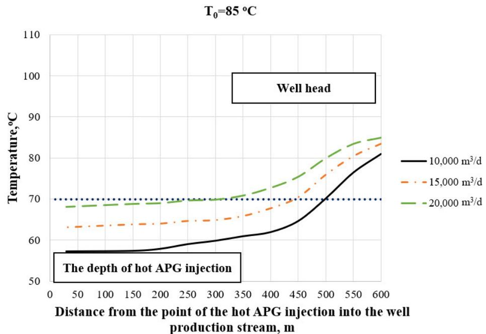
Figure 11. Annulus hot APG temperature profile, inlet  $T_0 = 85$  °C.
