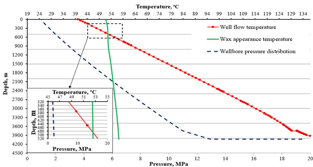
Figure 3. Determination of the depth of wax formation.
