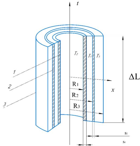
**Figure 1.** Pipe element during the injection of hot APG into the annular space of the well. 1—Tubing string; 2—Technological pipe (additional pipe); 3—Casing strings;  $T_1$ — Temperature of the injected APG in the space between the tubing string 1 and technological pipe 2;  $T_2$ — Temperature of the fluid inside the tubing string 1;  $T_3$ —Temperature of the fluid in the space between technological pipe 2 and casing strings 3.
