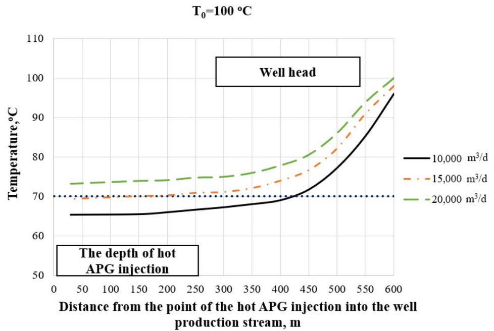
Figure 9. Annulus hot APG temperature profile, inlet  $T_0 = 100\text{ }^\circ\text{C}$ .
