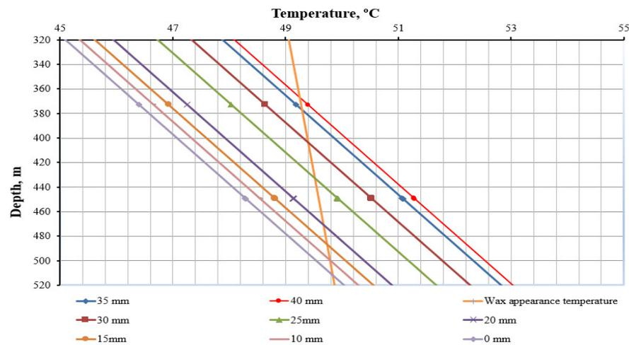
Figure 4. Selection of the optimal thickness of the heat-insulating polyurethane layers.
