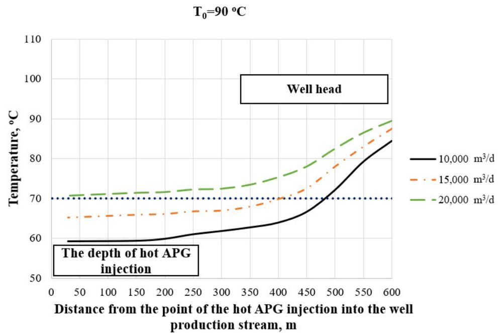
Figure 10. Annulus hot APG temperature profile, inlet  $T_0 = 90\text{ }^\circ\text{C}$ .
