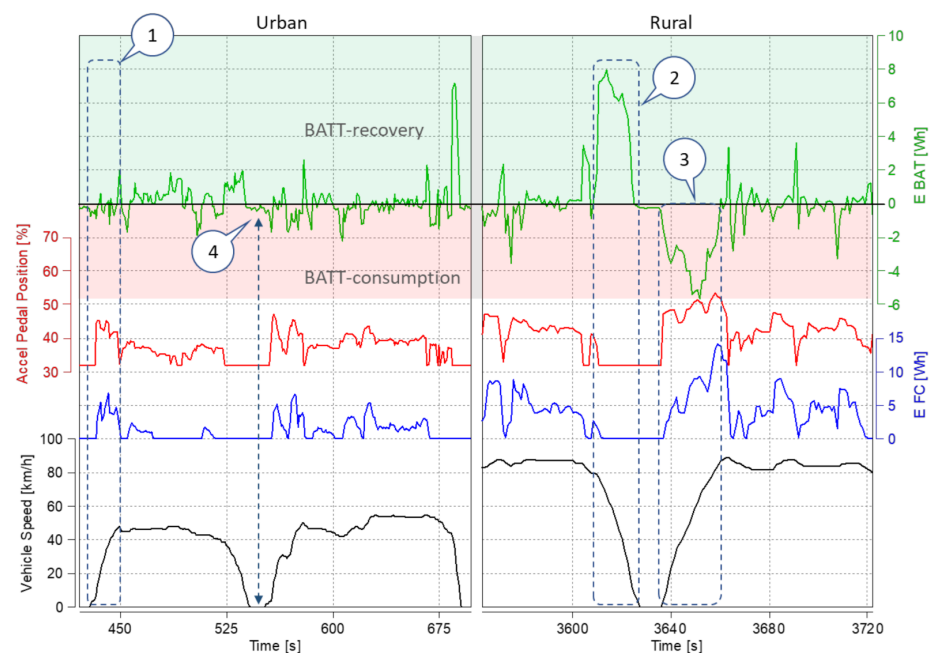
Figure 10. Interaction of powertrain components during driving of Toyota Mirai (selected events on road).
