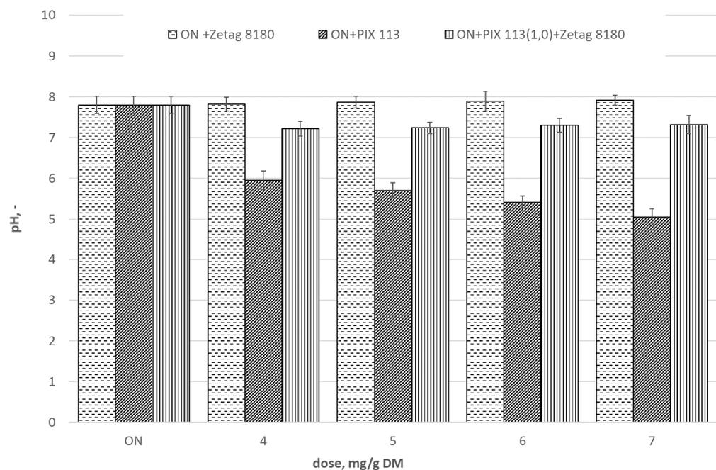
**Figure 7.** pH changes in filtrate after sludge dewatering. Sludge sonicated ( $A_1 = 15.25 \mu\text{m}$ ) and prepared with selected chemical reagents.
