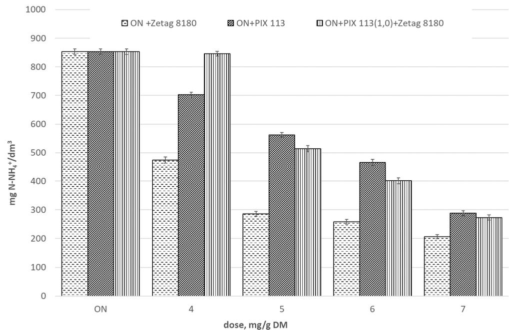
**Figure 10.** Ammoniacal nitrogen changes in filtrate after sludge dewatering. Sludge sonicated ( $A_1 = 15.25 \mu\text{m}$ ) and prepared with selected chemical reagents.
