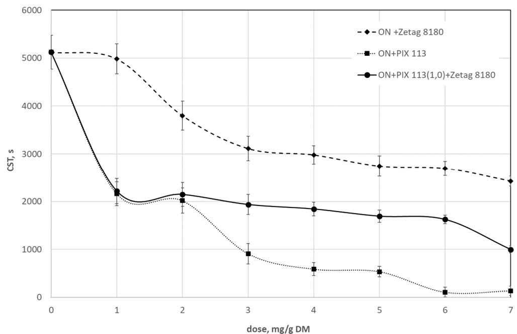
**Figure 2.** Effect of the dose of selected chemicals on CST of sonicated sludge ( $A_2 = 45.75 \mu\text{m}$ ).
