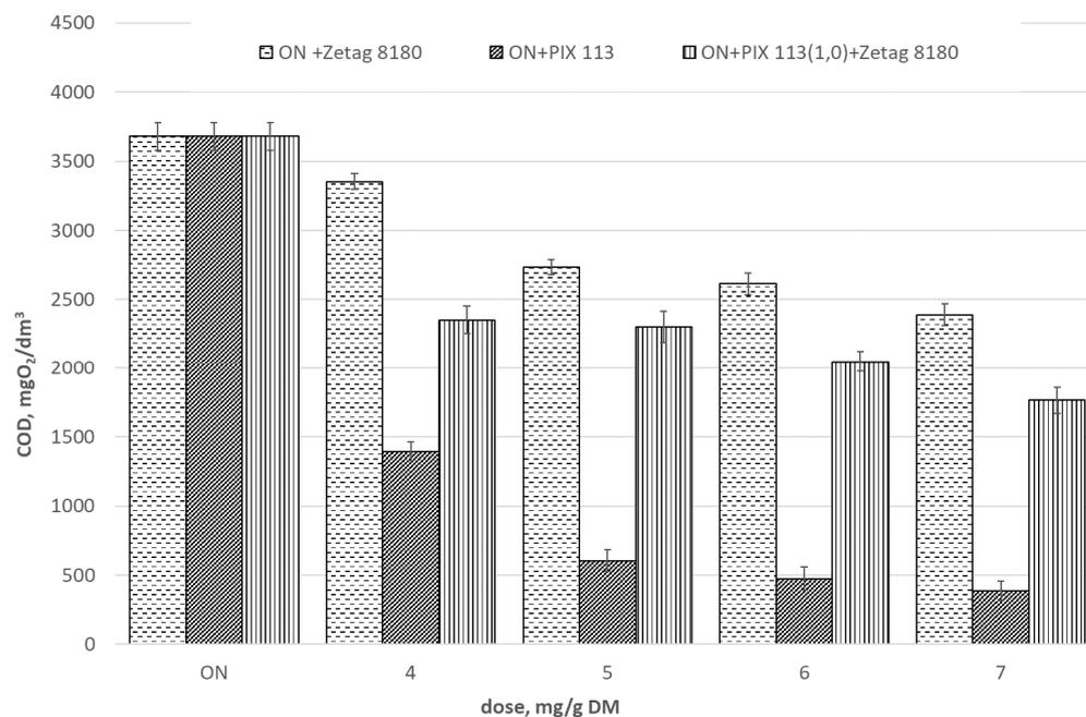
**Figure 8.** COD changes in filtrate after sludge dewatering. Sludge sonicated ( $A_1 = 15.25 \mu\text{m}$ ) and prepared with selected chemical reagents.
