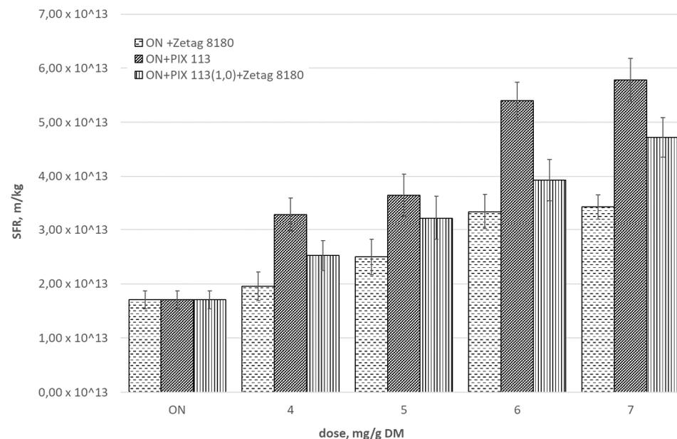
**Figure 4.** Effect of the dose of selected chemicals on SFR of sonicated sludge ( $A_2 = 45.75 \mu\text{m}$ ).
