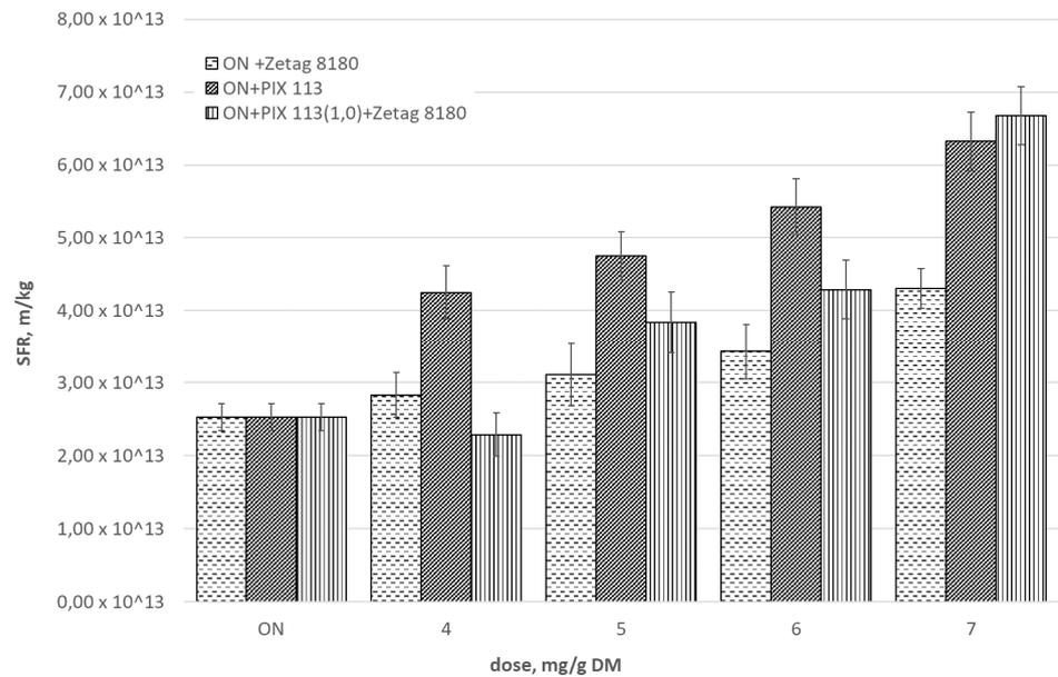
**Figure 3.** Effect of the dose of selected chemicals on SFR of sonicated sludge ( $A_1 = 15.25 \mu\text{m}$ ).
