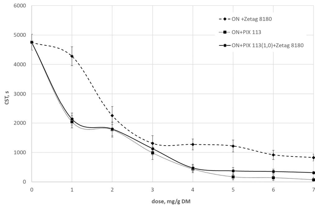
**Figure 1.** Effect of the dose of selected chemicals on CST of sonicated sludge ( $A_1 = 15.25 \mu\text{m}$ ).
