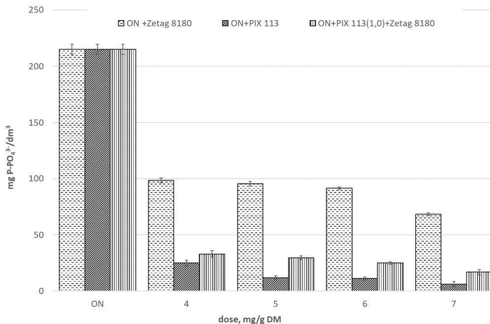
**Figure 9.** Phosphate changes in filtrate after sludge dewatering. Sludge sonicated ( $A_1 = 15.25 \mu\text{m}$ ) and prepared with selected chemical reagents.
