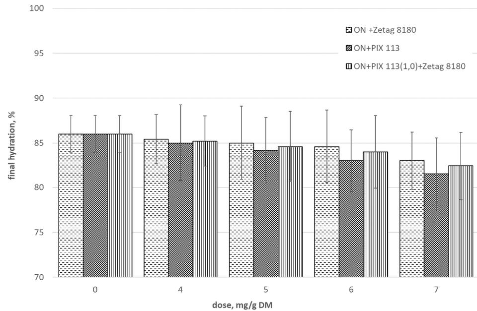
**Figure 5.** Effect of the dose of selected chemicals on the final hydration of prepared sludge ( $A_1 = 15.25 \mu\text{m}$ ).
