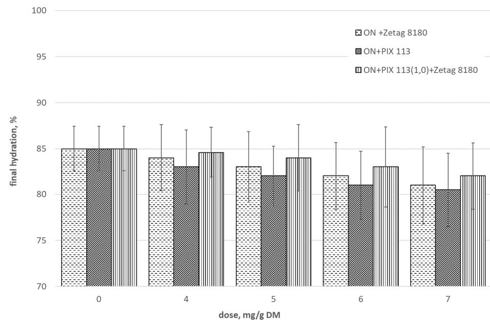
**Figure 6.** Effect of the dose of selected chemicals on the final water content of prepared sludge ( $A_2 = 45.75 \mu\text{m}$ ).
