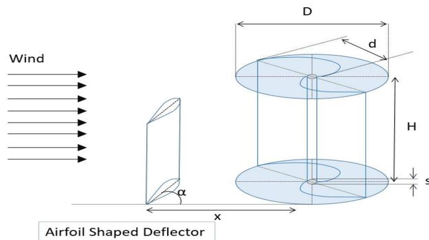
**Figure 6.** An airfoil-shaped wind deflector in the upstream of a Savonius rotor [75].
