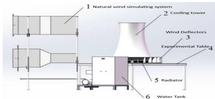
**Figure 12.** An experimental setup to investigate the effect of deflector in cooling tower [84].
