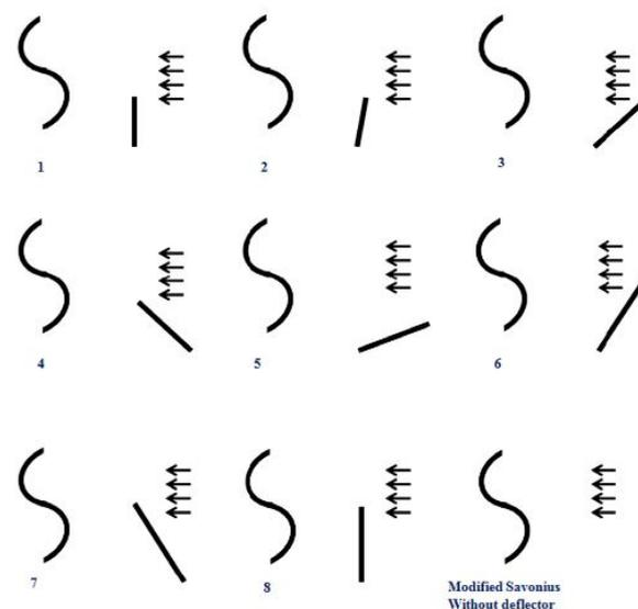
**Figure 7.** Various installation angles and positions of flat-plate deflectors (adapted from [20]).
