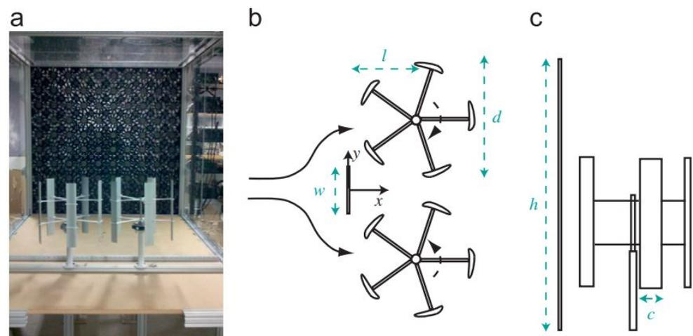
**Figure 10.** Wind deflector installed between two lift-based vertical axis wind turbines, (a) experimental setup in the wind tunnel, (b) top view, and (c) front view (adapted from [74]).
