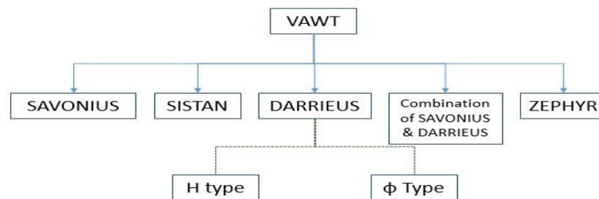
Figure 1. Classification of vertical axis wind turbines [22].
