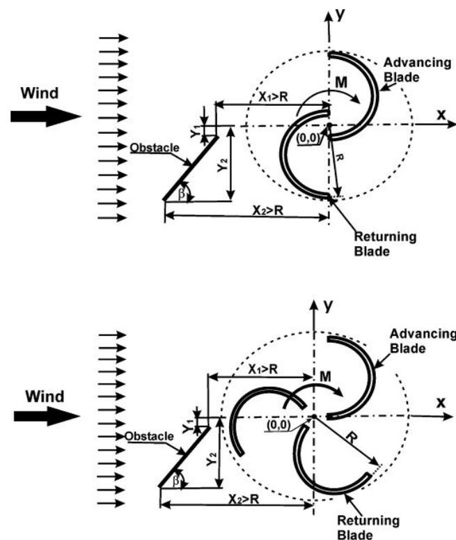
**Figure 8.** Power coefficient optimization of two-bladed and three-bladed Savonius turbine with flat-plate deflector (adapted from [77]).
