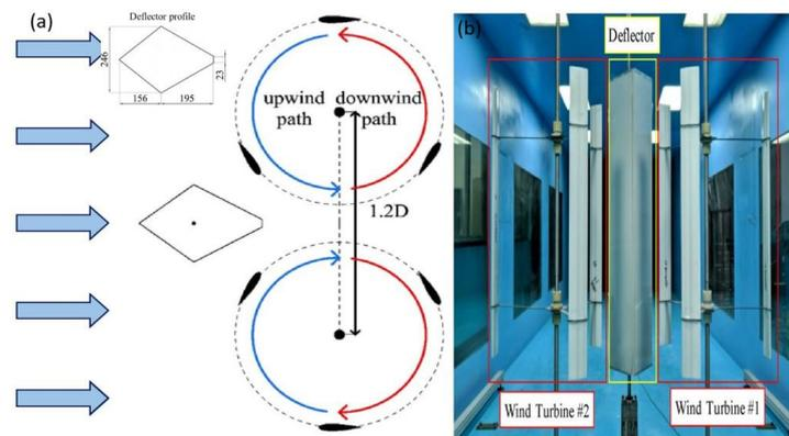
**Figure 11.** A kite-shaped wind deflector installed upstream of the VAWT. (a) Design. (b) Experimental test setup (adapted from [81]).
