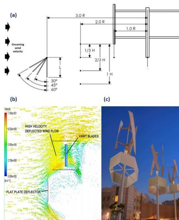
**Figure 9.** Flat-plate wind deflector in helical vertical axis turbine. (a) Design. (b) CFD analysis. (c) Installed deflector (adapted from [78]).
